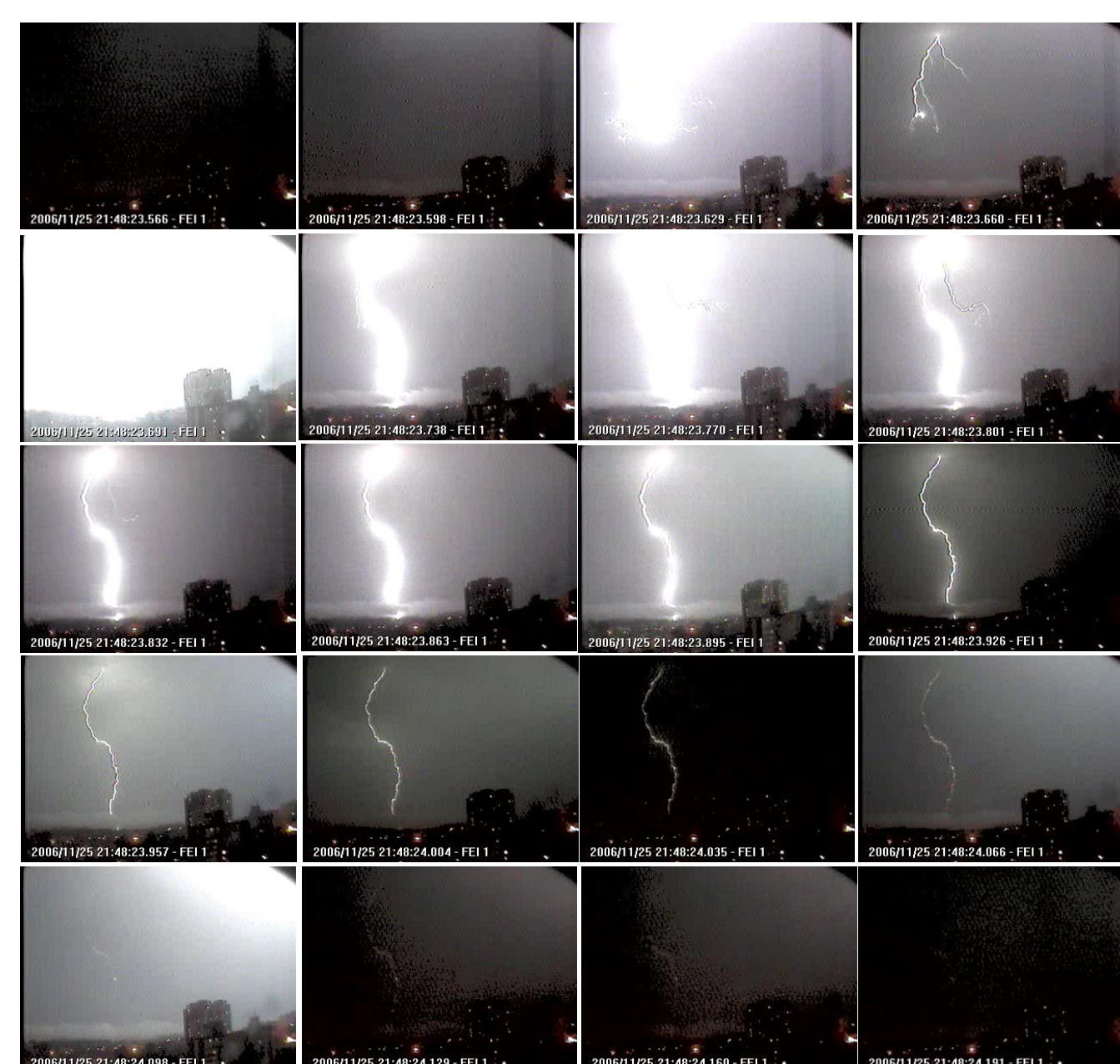
Figure 2: A lightning flash captured by the local monitoring system, occurred at SBC in 2006-11-25. The time interval between frames is 33,3ms.
