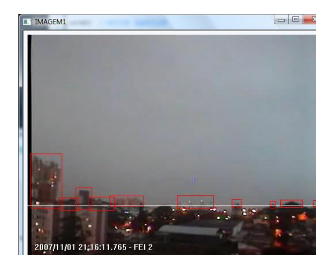
Figure 3: Image of a video camera. The red rectangles define obstacles and the white line defines the horizon line.
