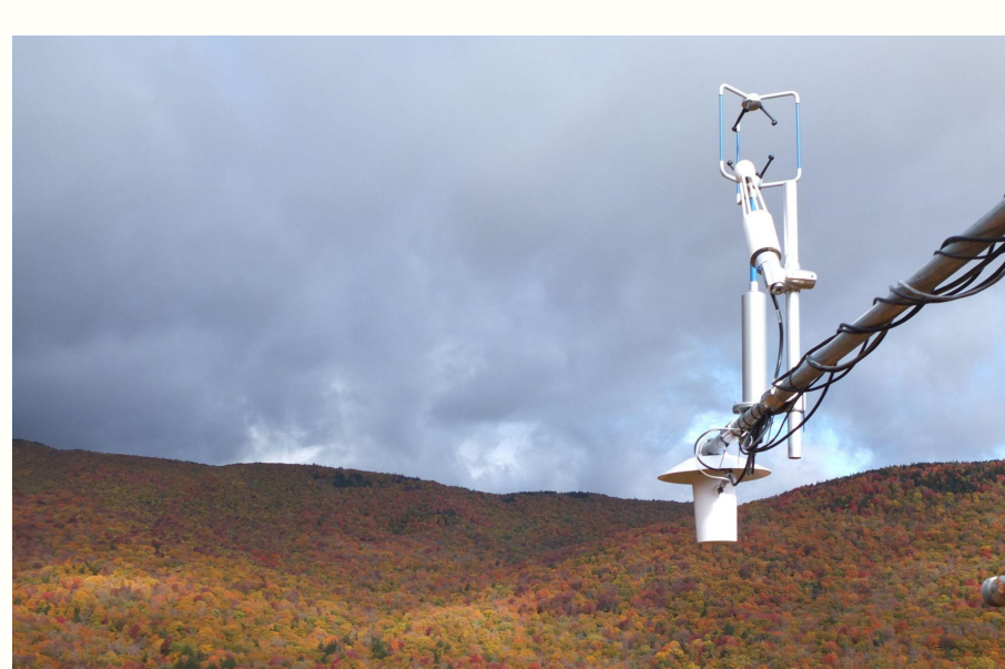
Figure 3. The above-canopy instrumentation on the eddy covariance tower in the HBEF (30 m agl).
