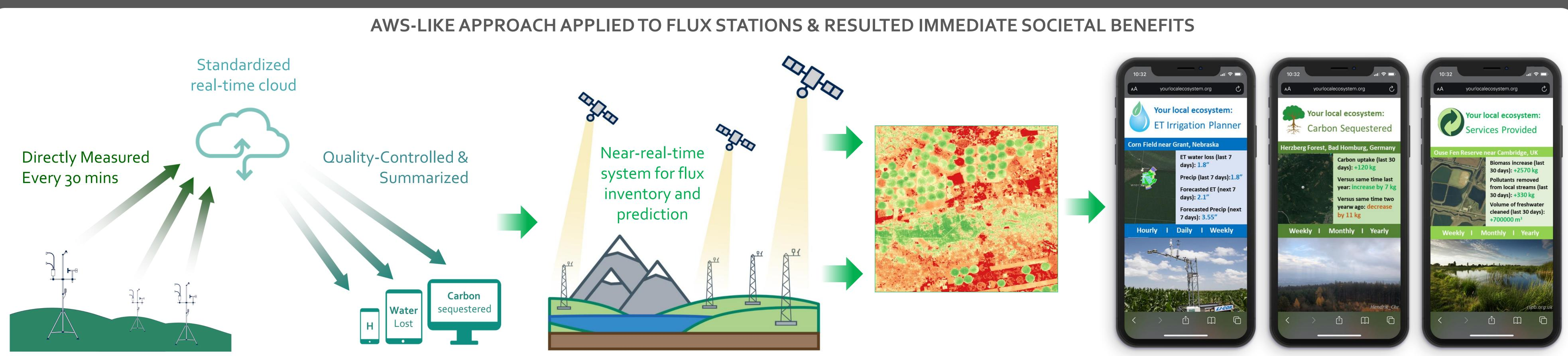
A future network of automated real-time flux stations (AFS) designed similar to the existing networks of automated weather stations (AWS), measuring GHG fluxes in addition to weather
