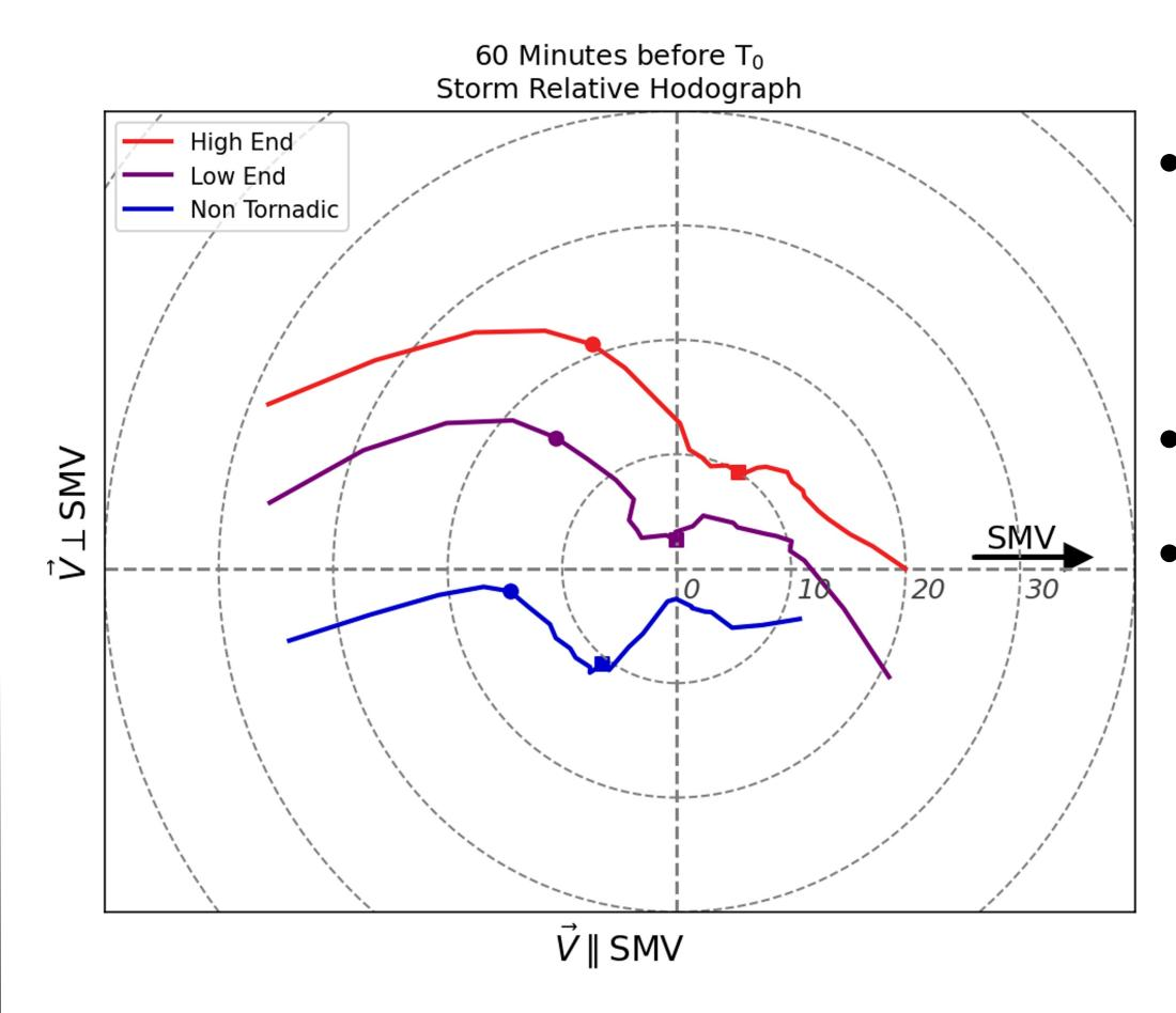
Using only NEXRAD data reveals differences between low end and high end tornadic QLCS environments. Higher end environments have stronger winds, as well as more veering in the low levels. As a result of this, shear and helicity are both higher.
