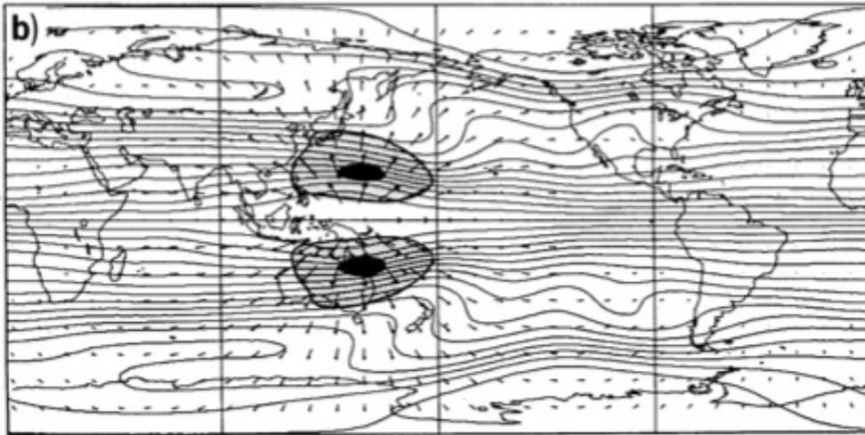
FIG. 2. (a) Rossby wave source  $S$  (shaded; units  $10^{-11} \text{ s}^{-2}$ ) on day 0. The steady divergent wind vectors and the initial absolute vorticity ( $10^{-9} \text{ s}^{-2}$ ) that determine this source are also shown. (b) as in (a) but on day 48 of the fully nonlinear integration. The largest divergent winds in the subtropics are about  $5 \text{ m s}^{-1}$ .
