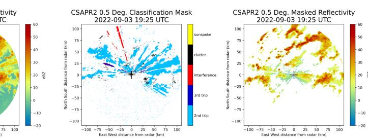
Interference is also identified in this PPI (red). Interference is caused by the radar waves interacting with another continuous wave, often associated with telecommunication links. These artifacts appear as radial spikes and are characterized by low SQI and high normalized standard deviation of received power.
