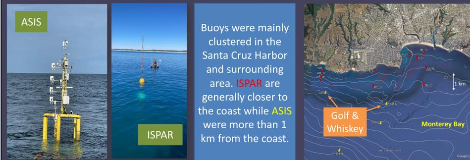
Photographs of an Air-Sea Interaction SPAR (ASIS) buoy (far left) and an Inner Shelf Spar (ISPAR) buoy (second from left) deployed over the Gulf of Mexico during a DRI CLASI Experiment in 2023. ASIS photo credit: Dr. Hans Graber, U. Miami; ISPAR photo credit: LCDR Charlotte Benbow, the Naval Postgraduate School.
