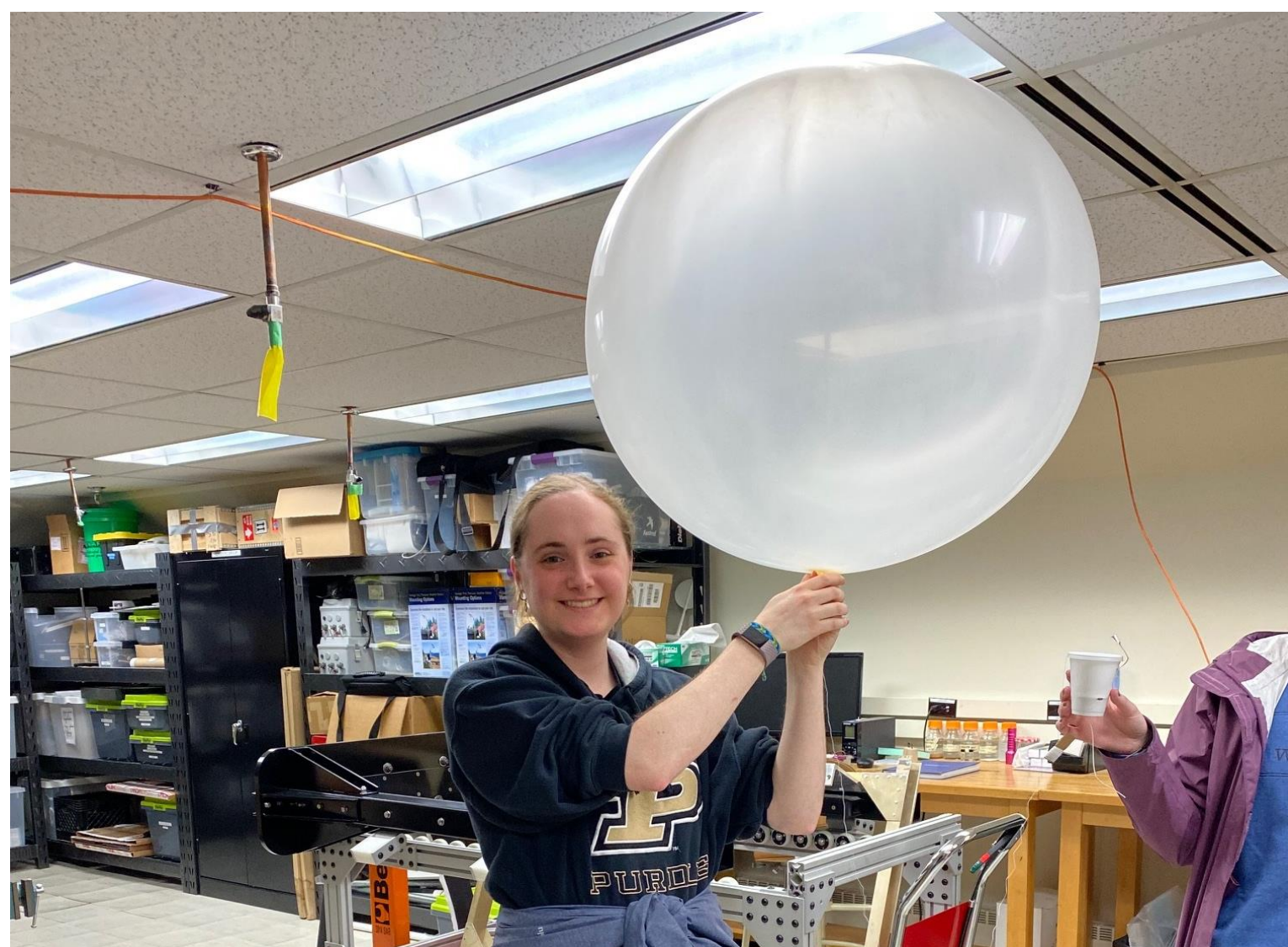
Fig. 1. The first author, holding a radiosonde (Windsond.com) that was launched 31 March 2023. The electronics in the cup to the right allow for data recording. Windonds have been used in meteorological research (Markowski et al., 2017).
