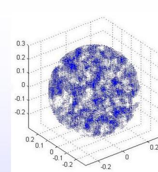
Figure 5. Computer prototype of a highly porous aerosol (HPA) composed of natural organic material (NOM), created by carving out voids of 0.03-microns radius using a random number generator. Axes are in units of microns. The refractive index of the filaments of NOM at wavelength 0.355 microns was taken to be  $1.60 + i0.14$  [Adler et al., 2014a,b].
