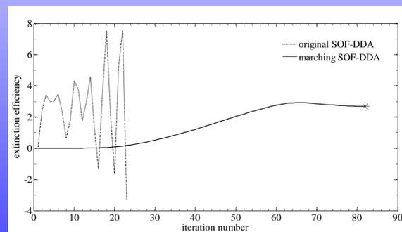
Figure 2. Successive values of extinction efficiency ( $Q_{\text{ext}}$ ) at wavelength 0.500 microns for a homogeneous water sphere of radius 0.3 microns with dipole spacing 0.01 microns, obtained using the original SOF-DDA model (dotted line) and the marching SOF-DDA model (solid line). The electric field of the incident radiation is polarized parallel to the scattering plane. Asterisk: theoretical value computed using the Mie scattering subroutine of Bohren and Huffman [1983, Appendix A].
