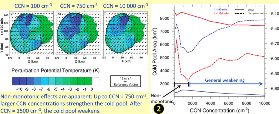
Non-monotonic effects are apparent: Up to  $\text{CCN} = 750 \text{ cm}^{-3}$ , larger CCN concentrations strengthen the cold pool. After  $\text{CCN} = 1500 \text{ cm}^{-3}$ , the cold pool weakens.
