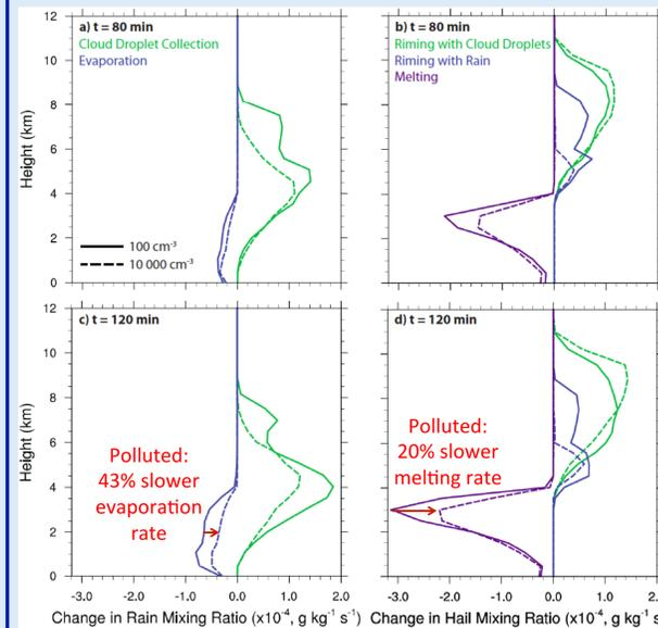
At larger CCN concentrations, evaporation and melting are reduced. Riming of hail with cloud droplets is increased.
