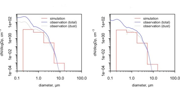
FIGURE 2. Simulated dust number concentration compared to surface measurements of aerosol number concentrations at Cape Verde Islands.
