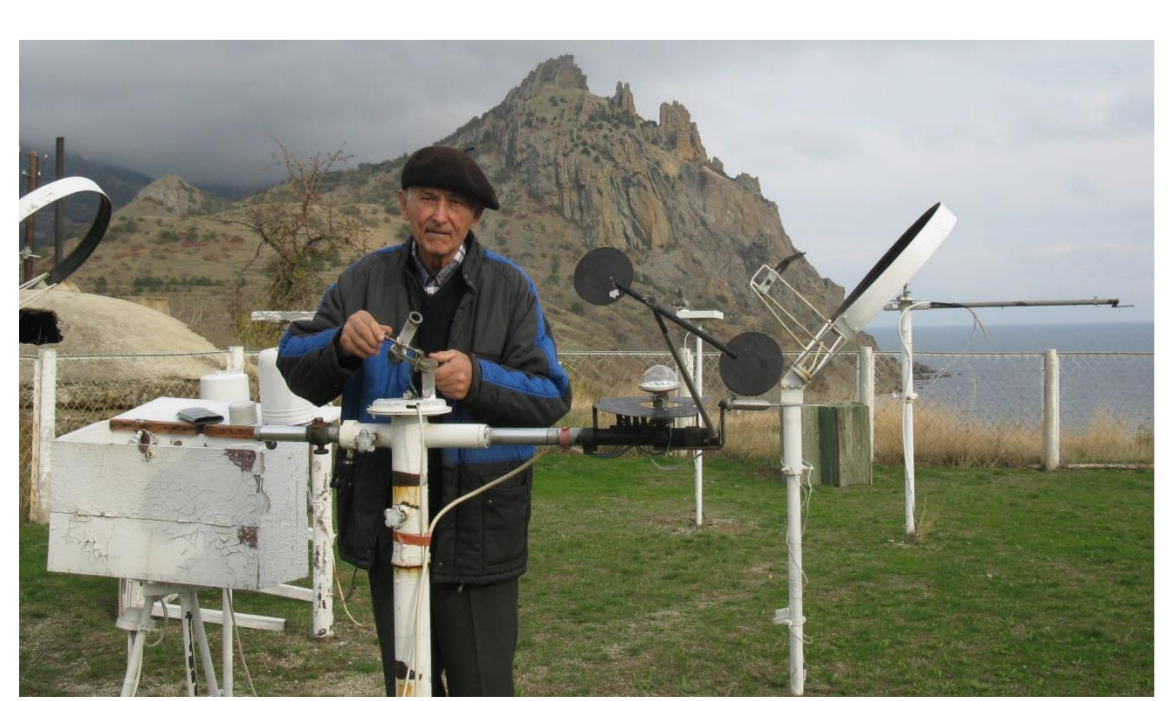
Fig. 3. For several decades G. Gushchin (PhD) has observed solar radiation in the Crimea.
