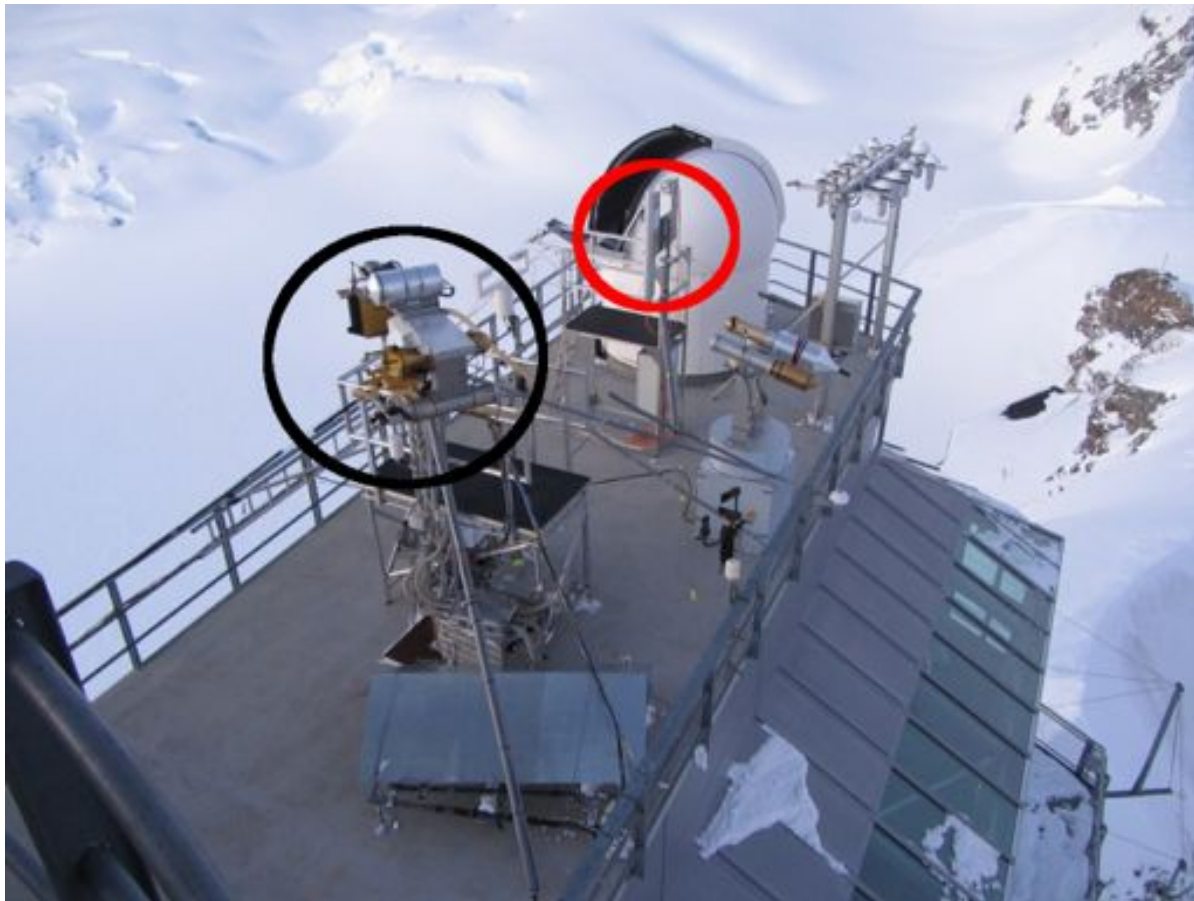
Figure 1: Location of the instruments used during CLACE2013. GipfelHolo is marked by a red circle, the instruments from the University of Manchester (which include the 2D-S) are marked with a black circle. The north-south line goes from the lower right to the upper left corner of the photo.
