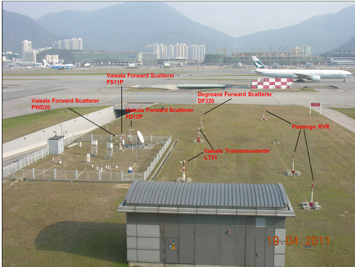
Figure 1 Setup of the visibility sensors under testing at the Hong Kong International Airport
