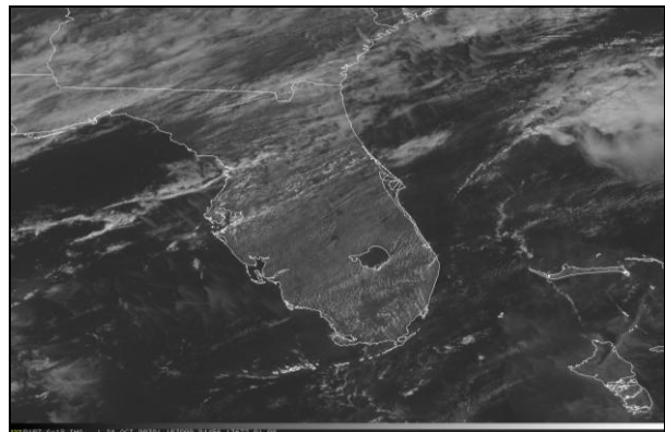
Figure 2. Satellite picture of the first Ares I-X launch attempt; high, thin clouds caused a violation of the triboelectrification rule within the Lightning Launch Commit Criteria, and the launch was scrubbed the first launch attempt.
