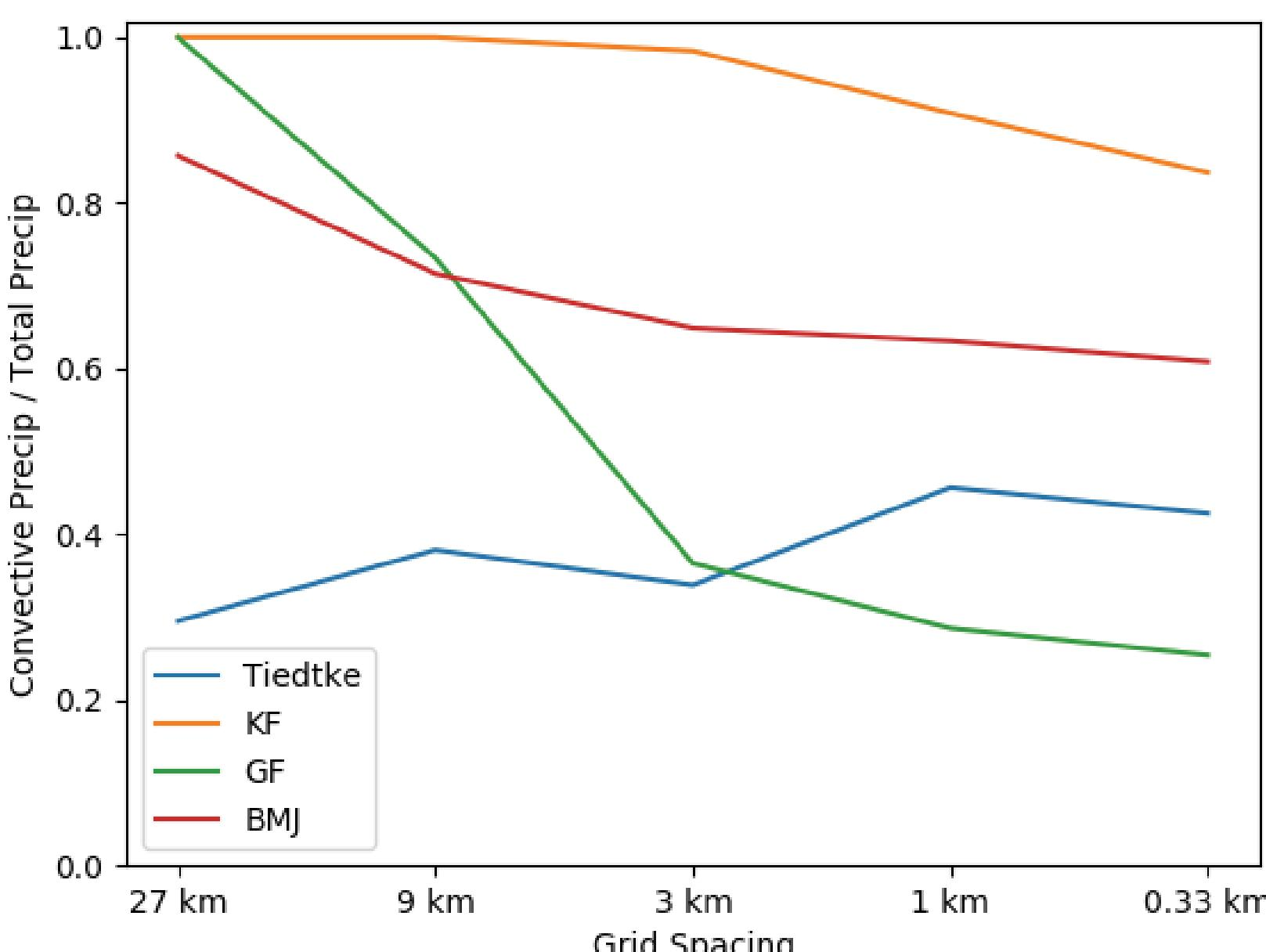
**Fig. 3:** Time and domain-averaged fraction of the convective over the total precipitation as function of grid length.
