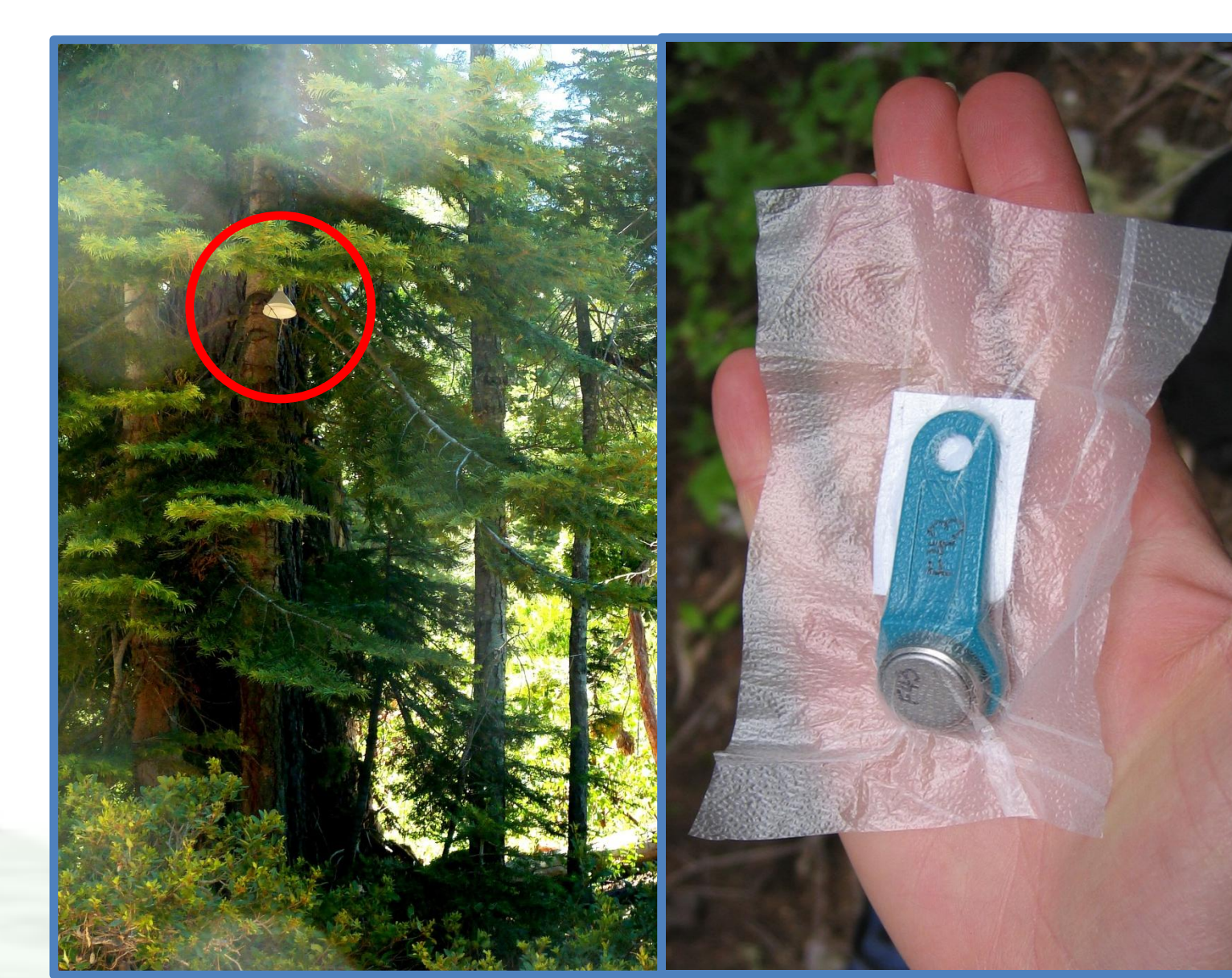
Fig. 3: iButtons for air (left) and ground temperature (right, before deployment) [4]
