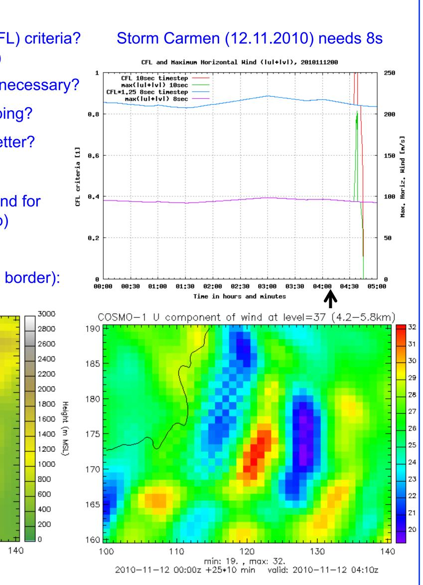
• The waves in the mid-troposphere (here from the NW) have a check pattern which do not depend on the choice of Rayleigh damping, diffusion or advection scheme used (other problem!)
