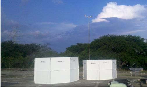
Fig.2: Main monitoring site ant Sub-Station Colima II, with SODAR/RASS and Aanderaa 10-m weather station in the background.
