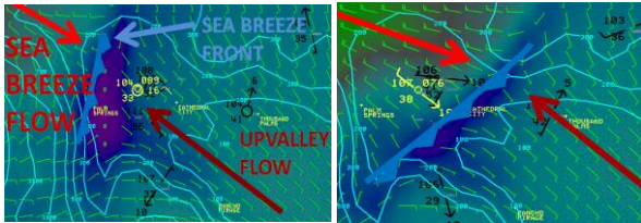
Fig. 1. The image on the left is the 15 hour forecast 1.5 km WRF-EMS ARW surface winds (green bars), wind speed (shading), and surface observations valid at 2100 UTC 12 August 2013. The leading edge of the sea breeze front is indicated (blue line with bars) and is seen quite well in the shading. Note the calm winds at Palm Springs (yellow METAR observation). Two hours later (at 2300 UTC 12 August 2013) the image on the right shows the sea breeze front has passed Palm Springs based on the model forecast and the observation, with gusts to 18 knots.
