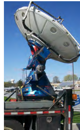
FIG. 2: The Doppler on Wheels operating during MEDOW IOP 1. The Millersville water tower is visible to the right above the tree line.
