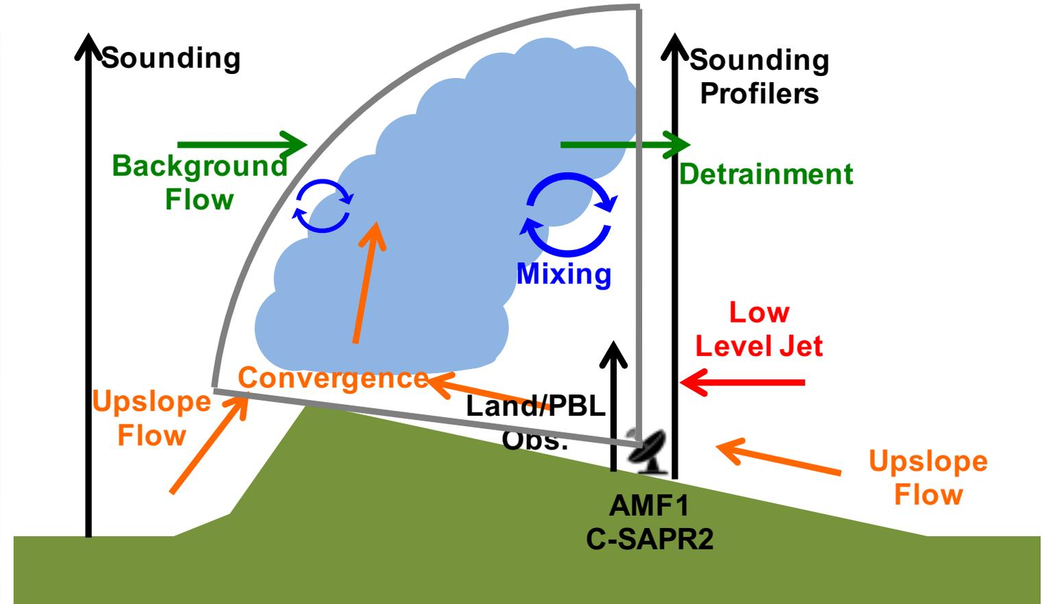
The goal was to measure cloud base inflow properties with in situ/remote sensing measurements of clouds, precipitation, and cloud-detained air properties in the free troposphere, with a focus on daytime operations and consistent measurements for many cases over the length of the campaign
