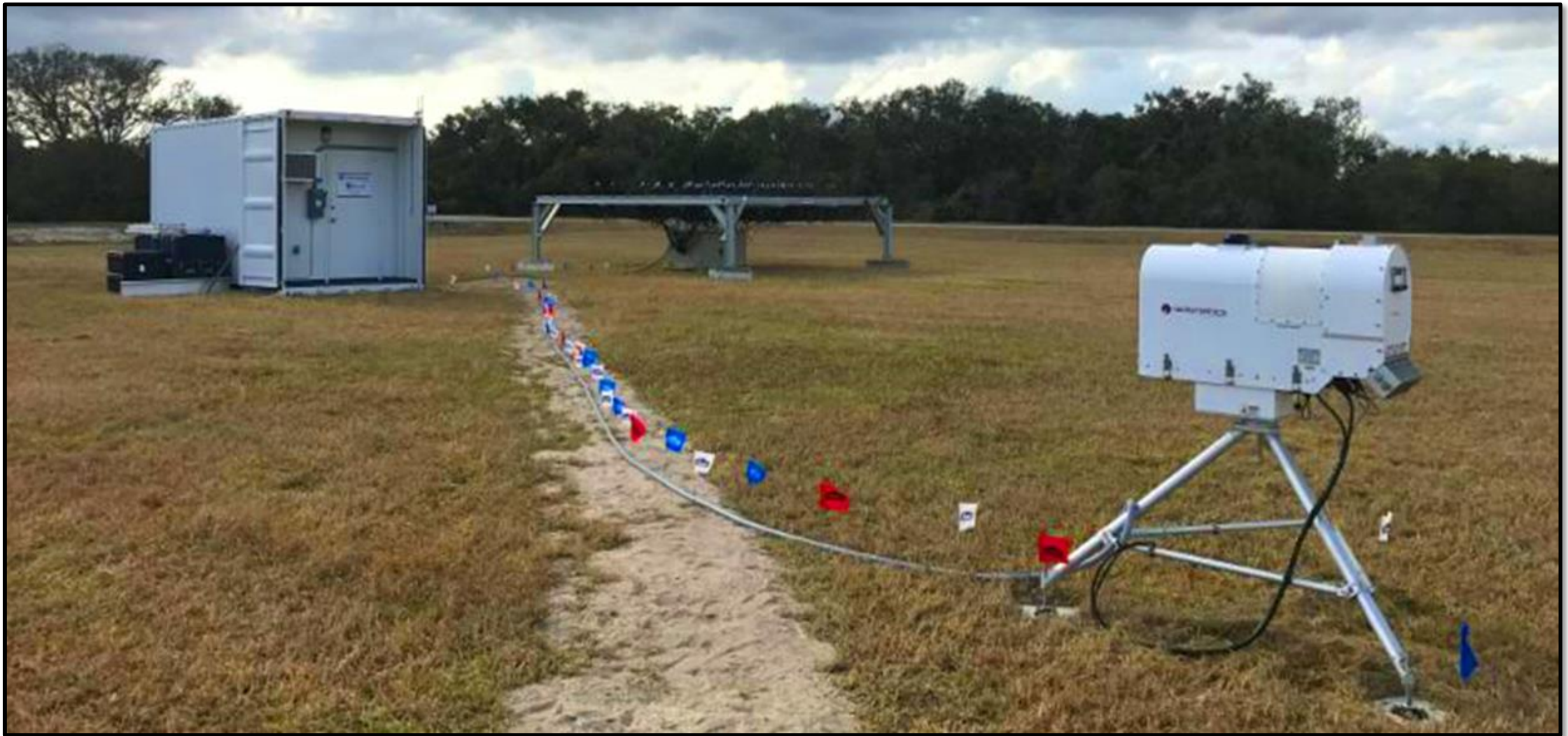
SkyCast ® wind (left) and thermodynamic (right) profilers at the Eastern Test Range (ETR).
