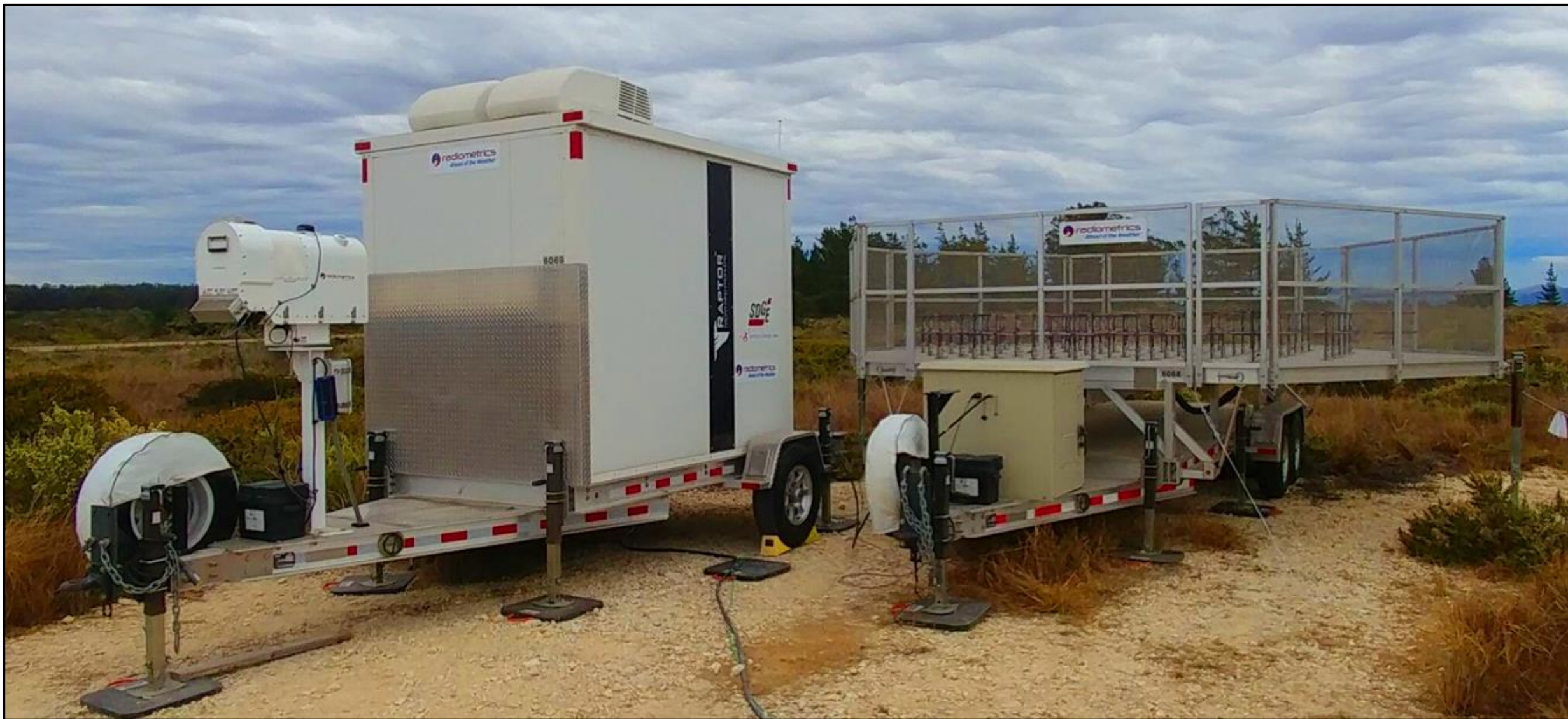
SkyCast® wind (right) and thermodynamic (left) profiler at the Western Test Range (WTR).
