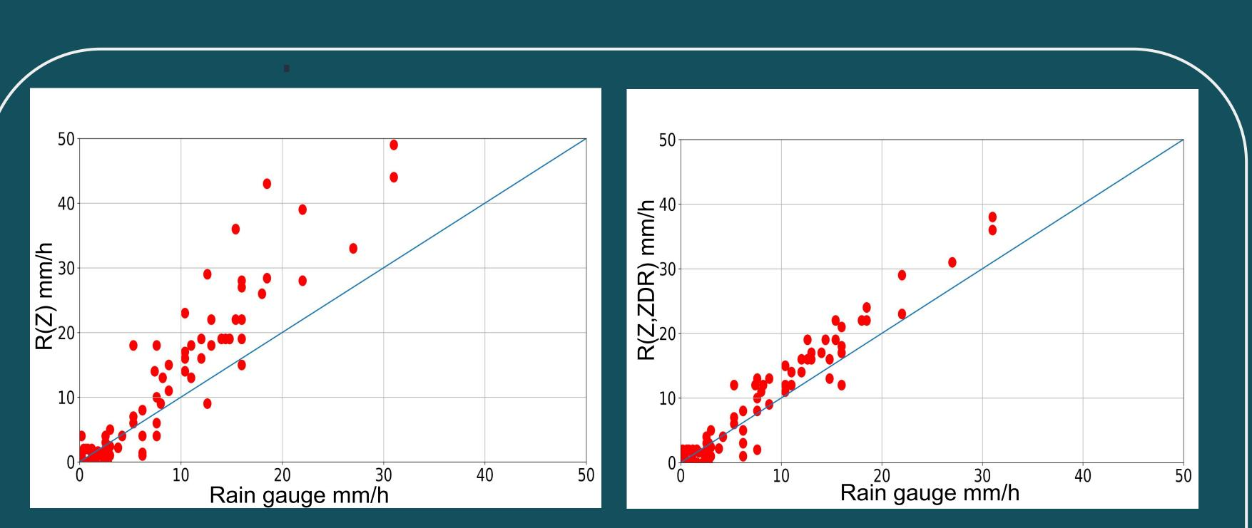
Hourly QPE as a reflectivity function(R(Z))(left) and reflectivity differential (R(Z,ZDR)) (right) for Jan-Aug 2018. The use of ZDR was important to adjust the QPE data.
