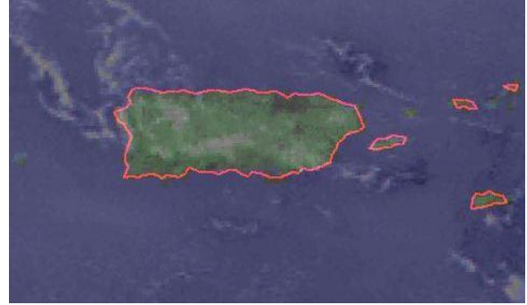
Figure 8d. Day/Night image for the same time as figure 8c. Note that some of the small clouds have been detected, but have been tinted blue like the water.
