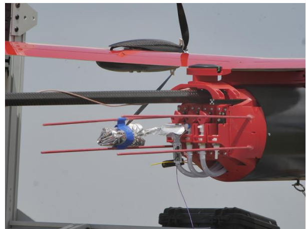
Figure 3: ALD in the storage position behind the fuselage of the Mistral before flight. Photo credit: Cole Kenny, IRISS.
