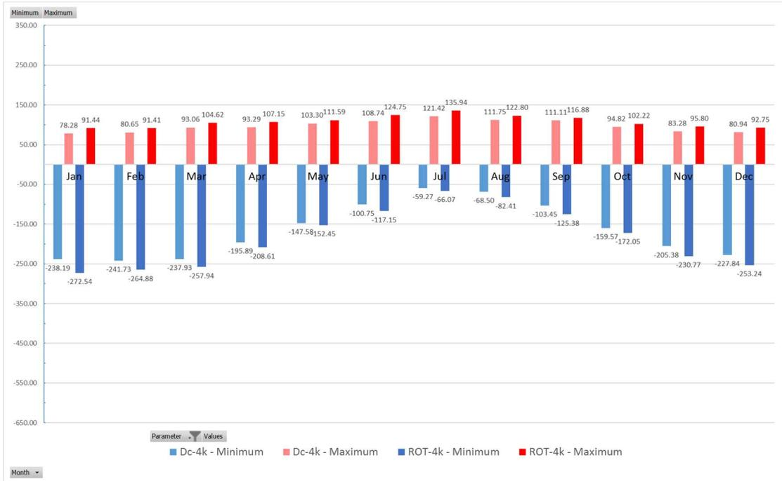
**Figure 1.** 30-year maximum (red) and minimum (blue) altimeter error at approximately 4 kft for entire model domain, calculated using both the corrected D-value and Rule of Thumb.
