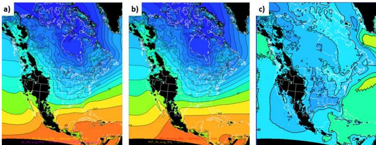
Figure 4. Calculation of altimeter error (m) at an approximate flight altitude of 4 kft using the corrected D-value (panel a) and the Rule of Thumb (panel b), while panel c shows the difference between the two. Negative (positive) values in panels a and c imply the aircraft is lower (higher) than indicated.
