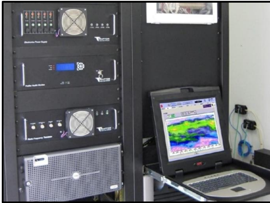
Figure 12. RAPTOR RWP control and data acquisition hardware.
