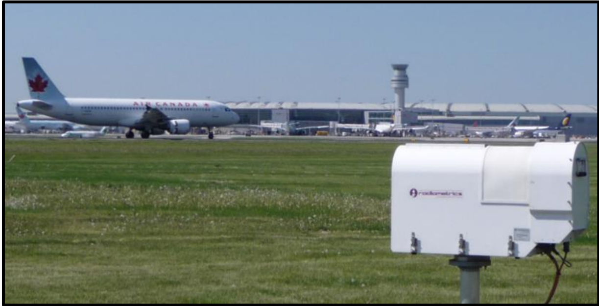
Figure 15. MP-3000A Microwave Profiler at Toronto Pearson International Airport (YYZ).
