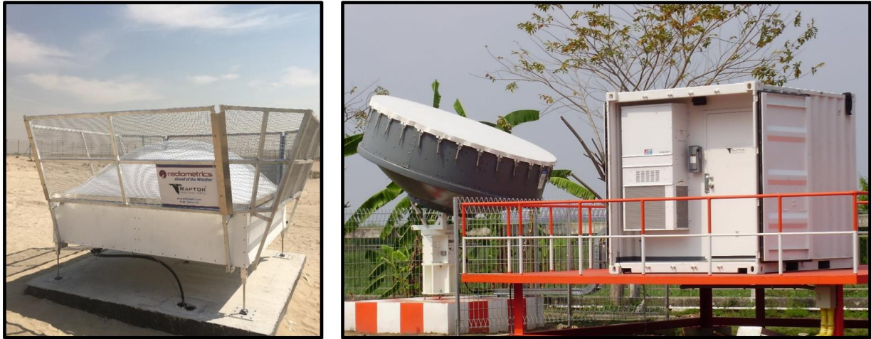
Figure 11. RAPTOR XBS-BL RWP phased array antenna (left) and VAD-BL (right).
