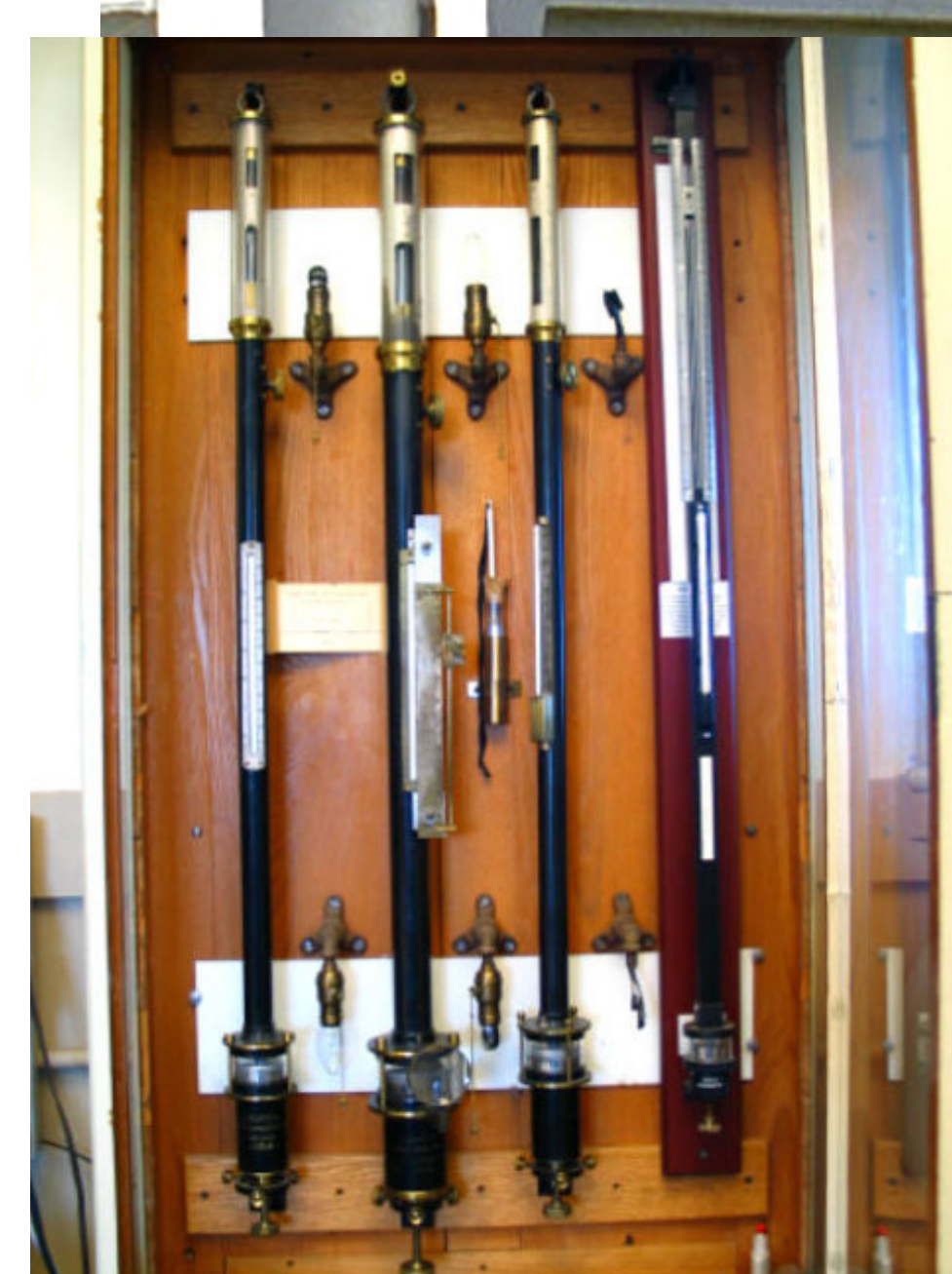
Mercury Barometers: Station Pressure
