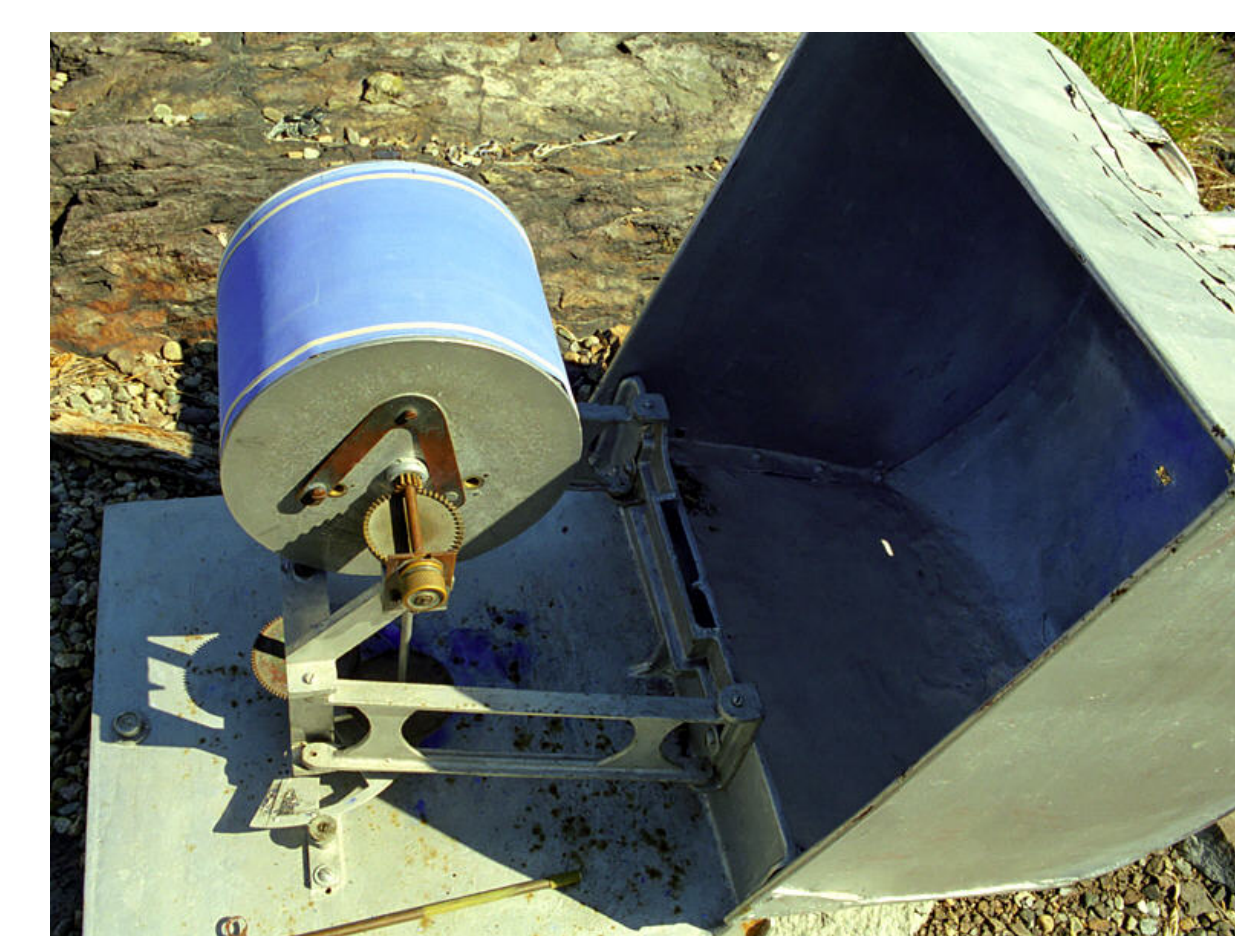
Ombroscope: Time of Precipitation
