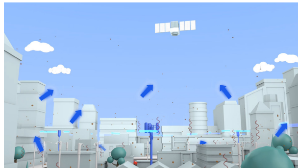
Figure 2: Upwelling adjacent band emissions and the natural upwelling signals from Earth and the atmosphere.
