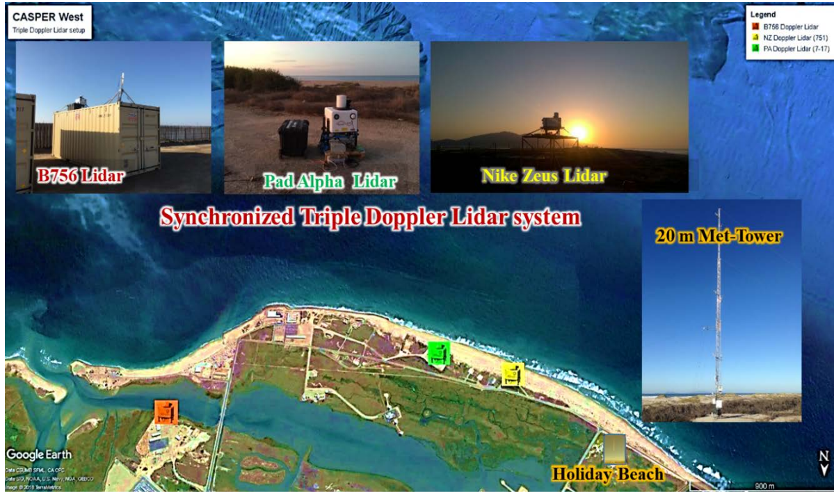
Triple Doppler Lidars at Point-Mugu + Flux Tower
