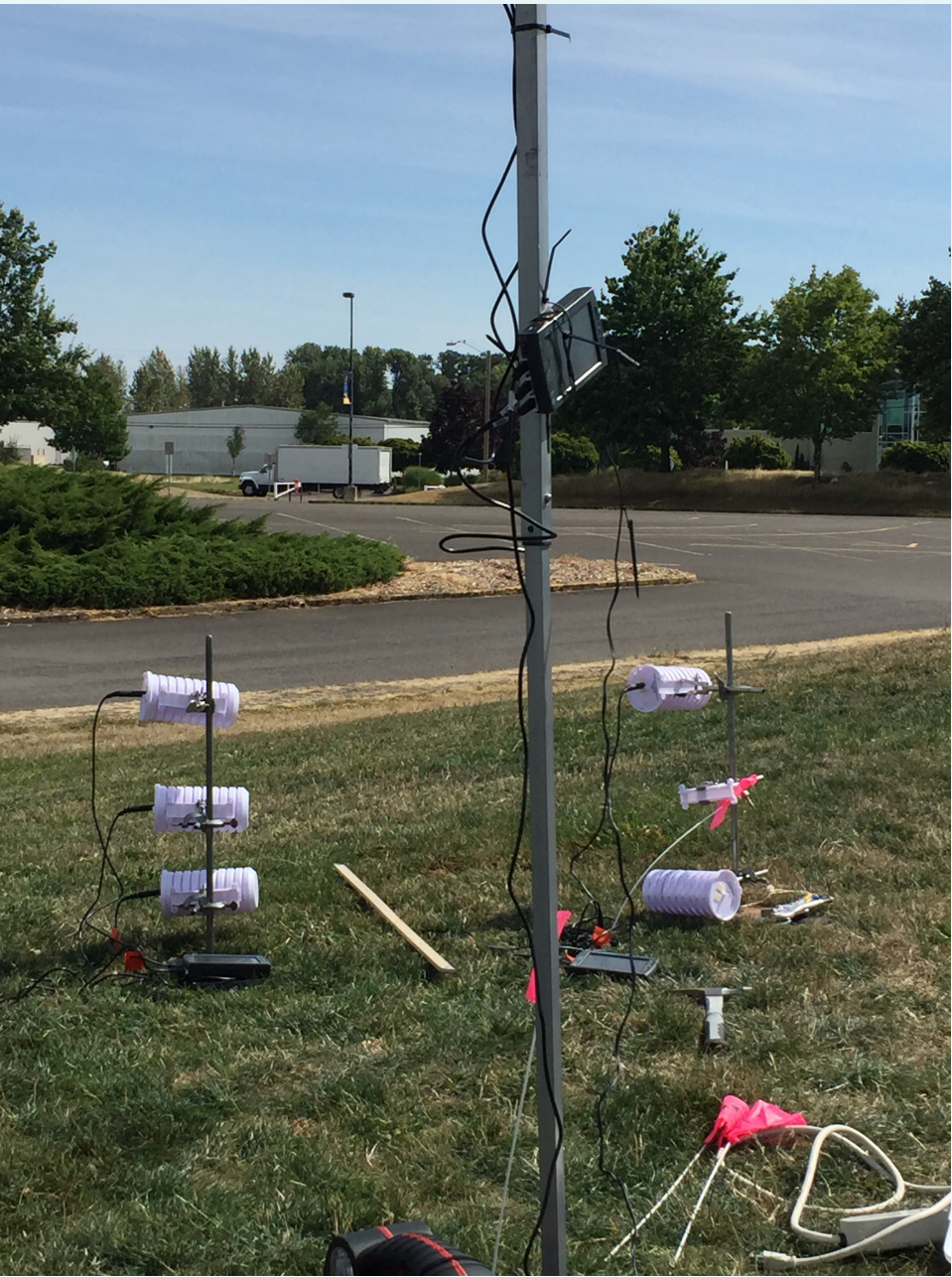
(Top) The near-surface instrument set-up at LBCC on eclipse day. Inexpensive thermistor radiation shields were used for all temperature and humidity recordings, along with Vernier probes and data loggers. Data were collected at 0.1 Hz during the event. (Bottom) – overall setup including “air” temperature and humidity station.
