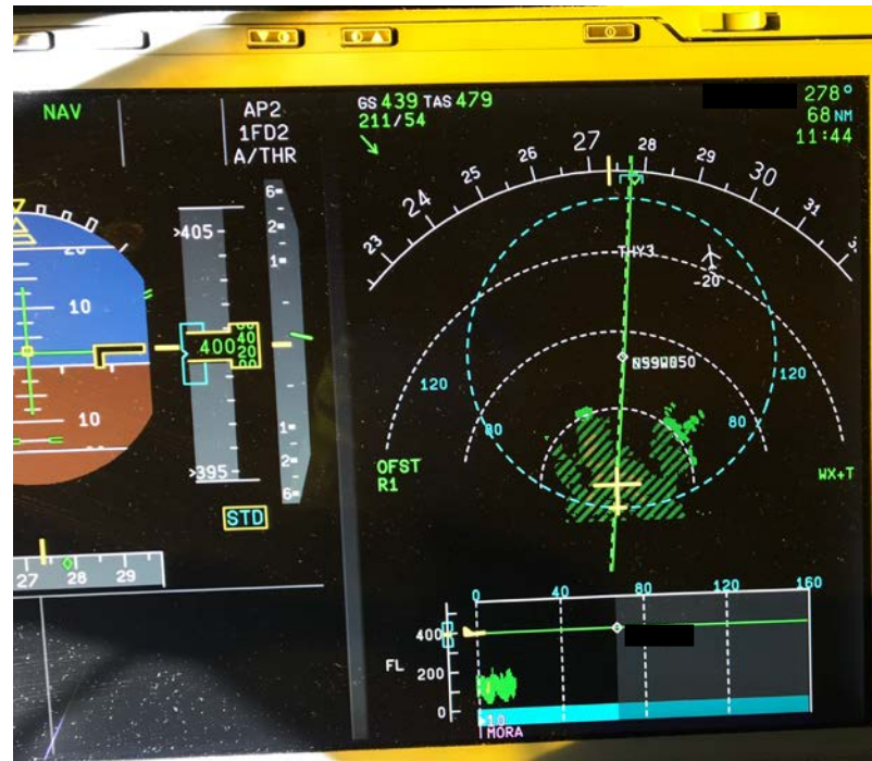
ND and WX RADAR at FL400 showing precipitation below our altitude. The hashed area indicates weather below FL250 along our route and the vertical display indicated the same.
