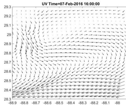
Fig.10 NSE ocean velocity field at  $t=0$
