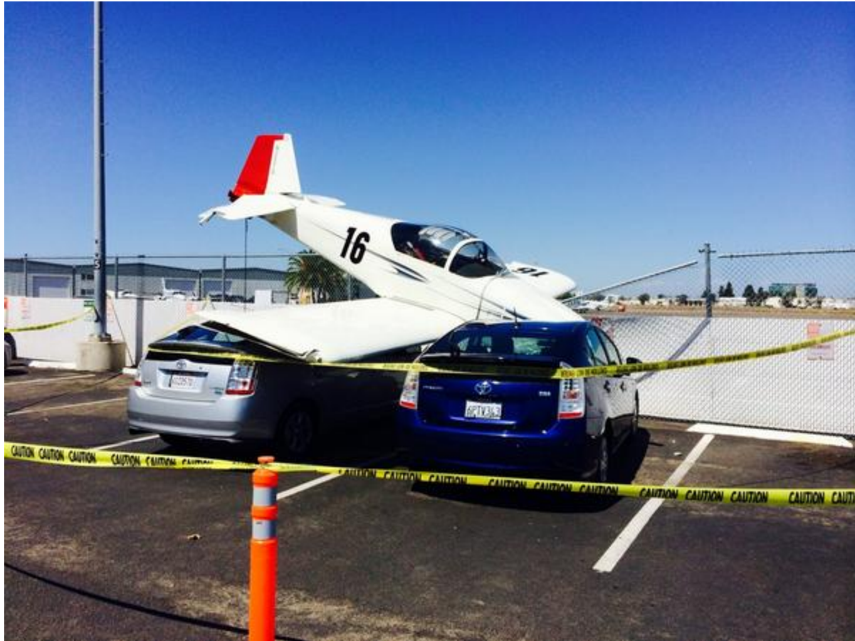
Figure 7a: Damage to airplane due to microburst
