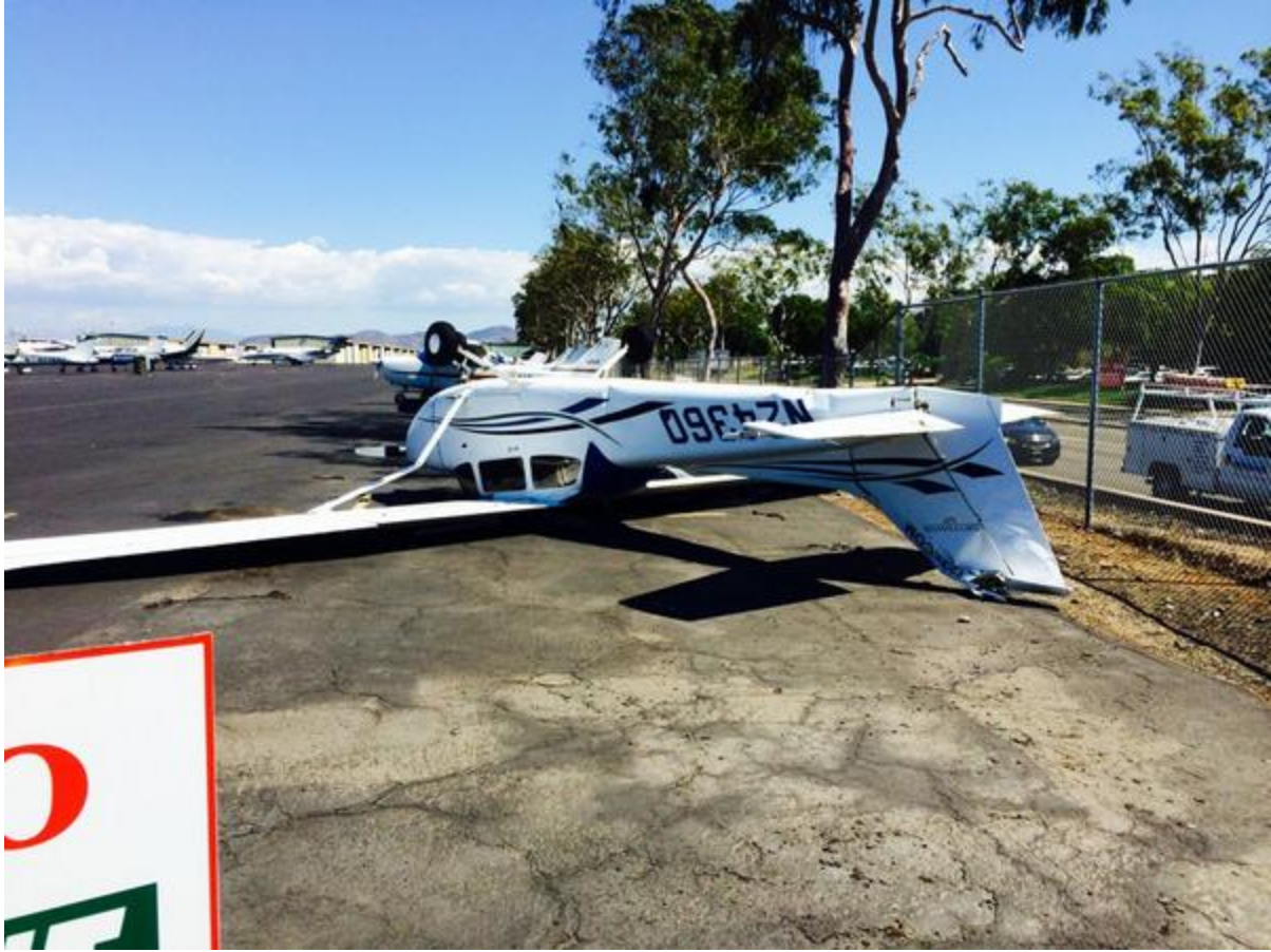
Figure 7b: Damage to airplane due to microburst at Montgomery Field
