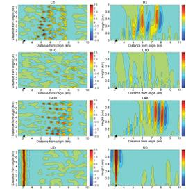
Left: Horizontal cross-sections of 500 m AGL vertical velocity (m s<sup>-1</sup>), 20 minutes after fire start. Right: Vertical cross sections of vertical velocity (m s<sup>-1</sup>) averaged in y-direction, 20 minutes after fire start. Note the different colorbar used for the U0 vertical cross section (bottom right panel). Fireline located 3.15 km from origin (see triangle symbol).
