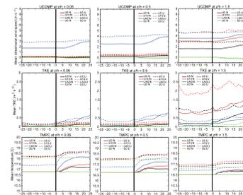
Timeseries of spatially averaged streamwise wind component (UOMP), turbulent kinetic energy (TKE), and temperature (TMPC), at surface (z/h = 0.06), mid-canopy (z/h = 0.5) and above canopy (z/h = 1.5). Fire start time indicated by vertical line.
