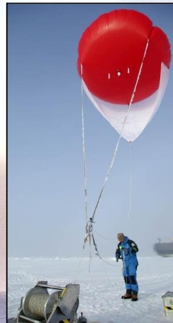
**Tethersonde: turbulent and mean sonde**
