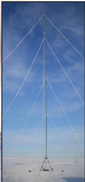
**Turbulence and micrometeorology masts (30m)**
