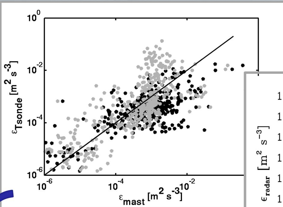
Comparison:  $\epsilon$  obtained with the sonic anemometer in the mast @ 30 m (black dots) and @ 15 m (gray dots) and  $\epsilon$  obtained with tethersonde
