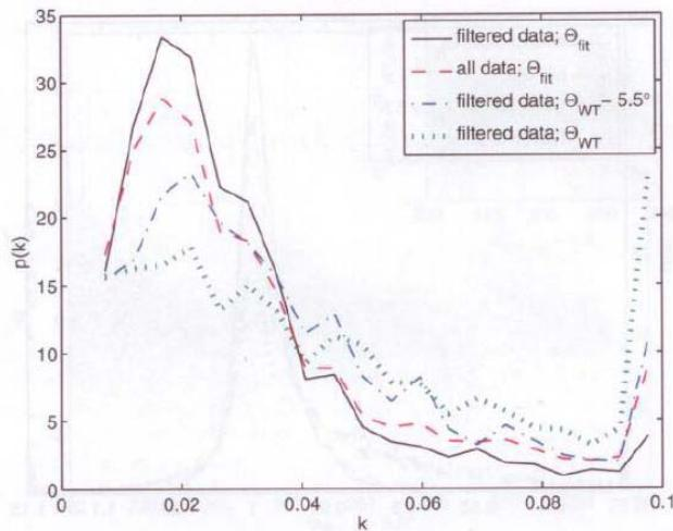
Figure 8. Distribution  $p(k)$  of wake-decay parameters obtained from best fit to all (f1)-(f3) filtered 10 min events (solid), best fit to all, i.e. non-filtered, 10 min events (dashed), one-parameter fit to all (f1)-(f3) filtered 10 min events with pre-assigned wind direction  $\Theta = \Theta_{WT} - 5.5^\circ$  (dash-dotted) and one-parameter fit to all (f1)-(f3) filtered 10 min events with pre-assigned wind direction  $\Theta = \Theta_{WT}$  (dotted)
