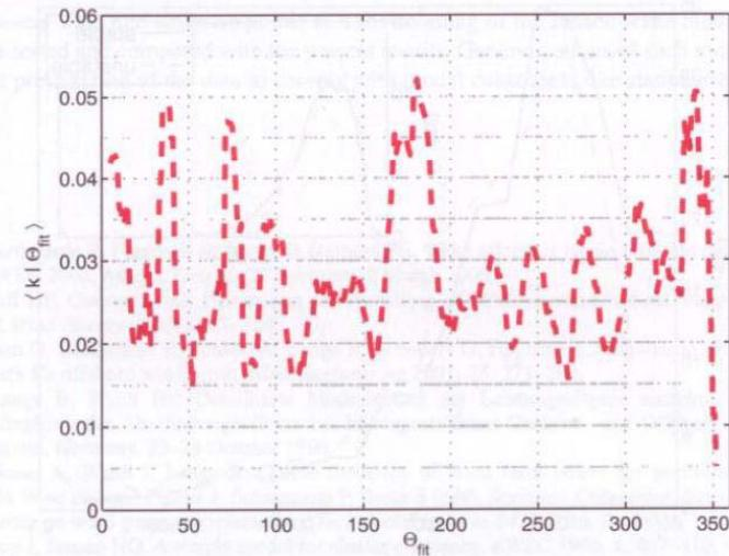
Figure 9. Wake-decay parameter  $k$  apportioned on the wind direction  $\Theta_{fit}$ . The conditional average  $\langle k | \Theta_{fit} \rangle$  (thick red line) is calculated as a moving average with  $10^\circ$  width
