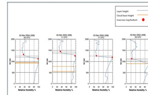
Figure 9. Relative humidity soundings from November 3, 2004; the top and bottom of the inversion are marked with red dots. The horizontal orange lines represent the ceilometer cloud bases and the dashed gray line represents the height of the layer of enhanced profiler reflectivity.
