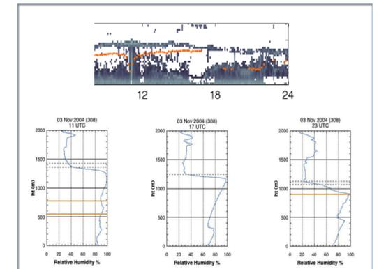
Figure 10. Closeup of data from November 3, 2004, showing a secondary inversion. At 11 UTC, an inversion is apparent at around 300m; it rises to 400m by 23 UTC.
