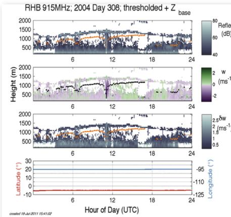
Figure 7. Thresholded profiler reflectivity, vertical velocity, and spectral width from November 3, 2004, overlotted with ceilometer cloud base heights (black or orange dots).
