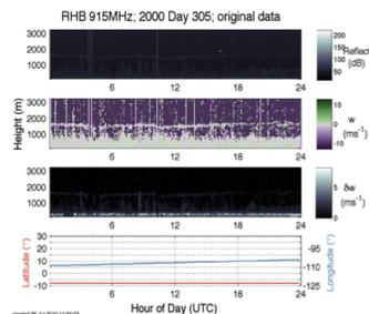
Figure 4. "Raw" profiler data from November 1, 2000: the vertical beam's reflectivity, vertical velocity, and spectral width as functions of time and height, together with ship position.
