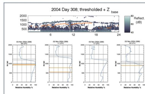
Figure 8. Thresholded profiler reflectivity for November 3, 2004, together with the corresponding humidity soundings. The horizontal orange lines in the soundings represent the ceilometer cloud bases and the dashed gray line represents the height of the layer during the time it took the radiosonde to ascend to about 3km.
