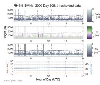
Figure 5. "Thresholded" profiler data from November 1, 2000: the vertical beam's reflectivity, vertical velocity, and spectral width as functions of time and height, plus ship position.
