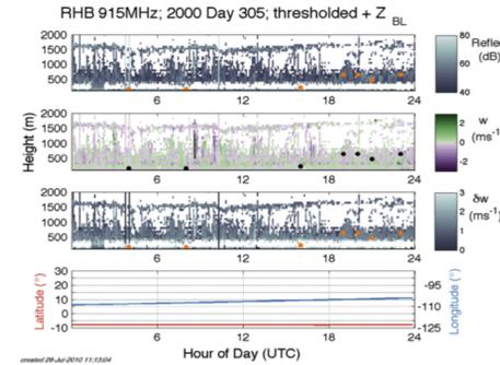
Figure 6. "Thresholded" profiler data from November 1, 2000 (reflectivity, vertical velocity, and spectral width) as functions of time and height. Colored dots indicate BL heights estimated hourly with a modified version of the Bianco et al. (2008) algorithm.
