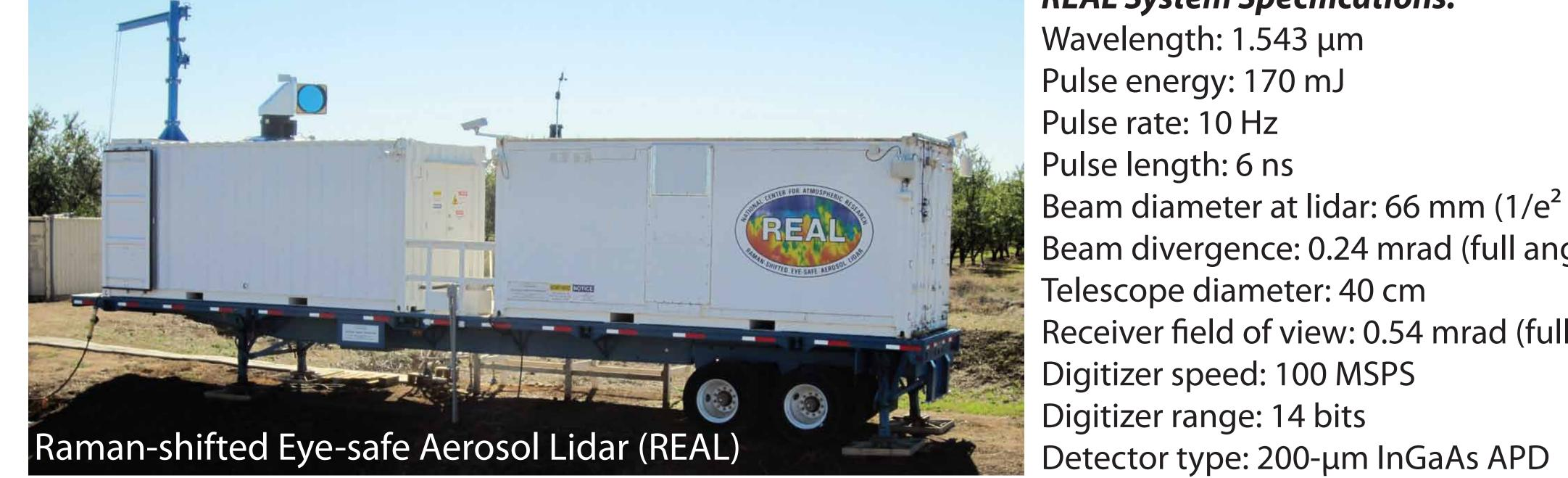
**REAL System Specifications:** Wavelength: 1.543 µm Pulse energy: 170 mJ Pulse rate: 10 Hz Pulse length: 6 ns diameter at lidar: 66 mm  $(1/e^2 \text{ points})$ Beam divergence: 0.24 mrad (full angle) Telescope diameter: 40 cm Receiver field of view: 0.54 mrad (full angle) Digitizer speed: 100 MSPS
