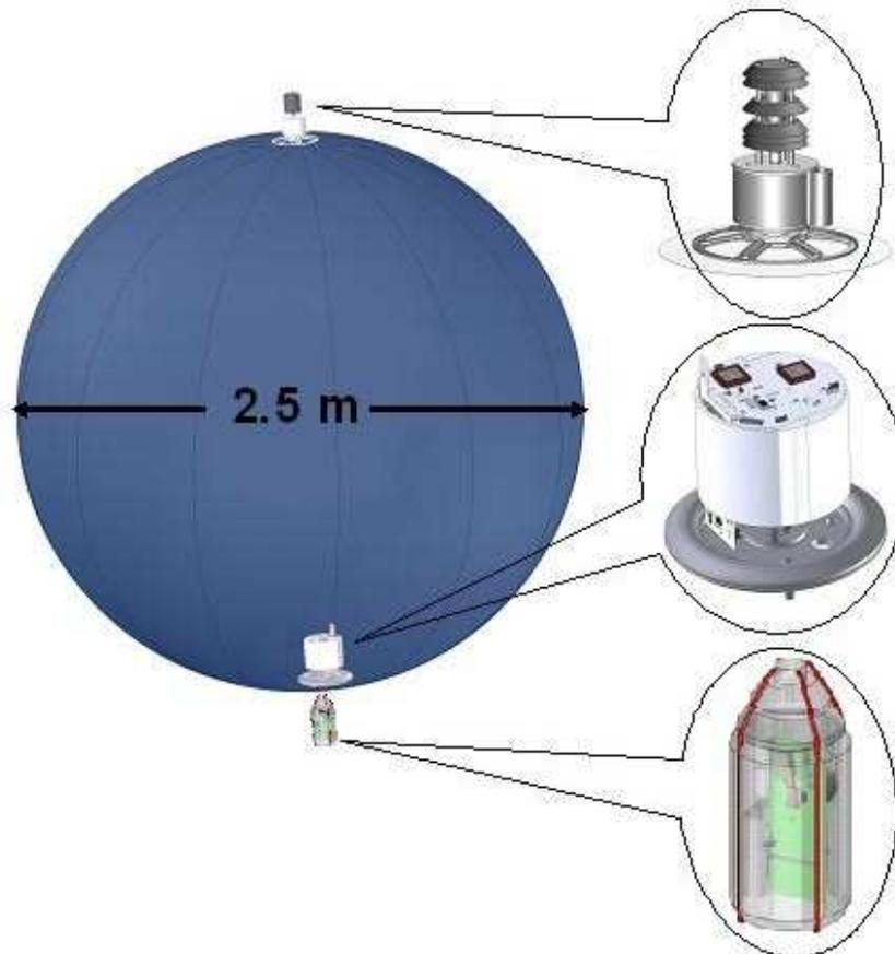
*Figure 1: The BLPB envelope, with the generic instrumentation (on the top), the system gondola (inside the envelope) and the additional instrumentation (on the bottom).*
