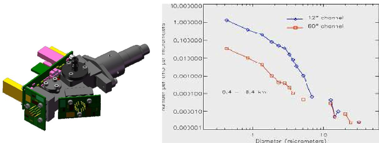
Figure 3: Model of the LOAC system (left) and example of aerosol size distribution observed at the two light scattering angles (right). The 12-deg channel is relatively insensitive to the refractive index and is calibrated in size, whereas the ratio between the two channels provides an indication of the nature of particles.
