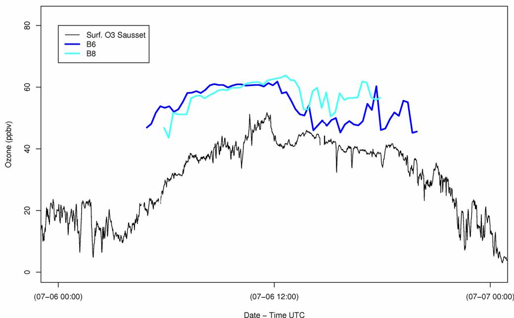
Figure 6: Time series of ozone mixing ratio on July 6 measured at ground level on the launch site (lower black curve) and during two BLPBs flights at about 500 m above the sea (upper curves).
