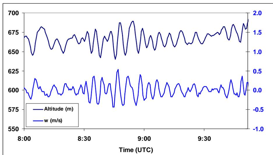
Figure 5: Example of BLPB oscillation in a gravity wave field. The time series of the BLPB altitude (black upper curve, left scale) and the corresponding BLPB vertical velocity (blue lower curve, right scale) are
