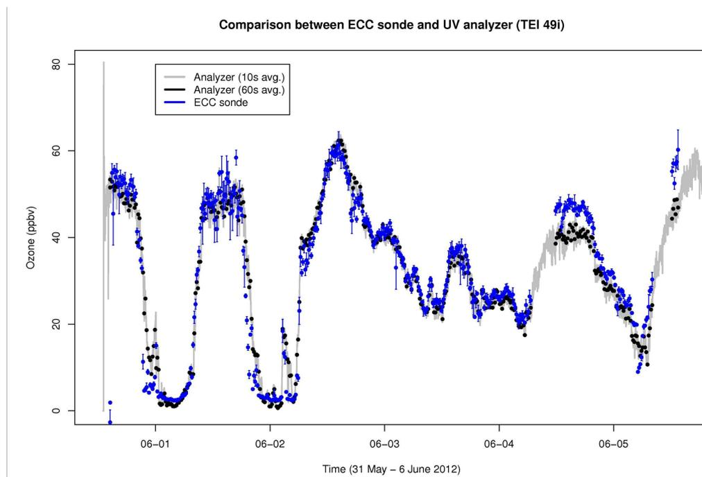
Figure 2: Time series on a 6-day period of the ozone concentration measured by a UV analyzer (at 10-s and 1-min average, gray and black dots, respectively), and the intermittent ECC sonde (blue).
