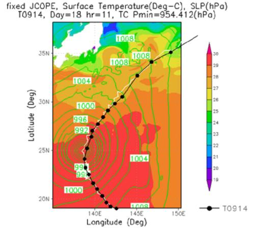
Figure 4. Sea level pressure (green contours), the SST distribution (colored) and the tracks in the experiment of the fixed SST (white line) at 60 hour of the integration time. Black line with dots shows the JMA Besttrack.
