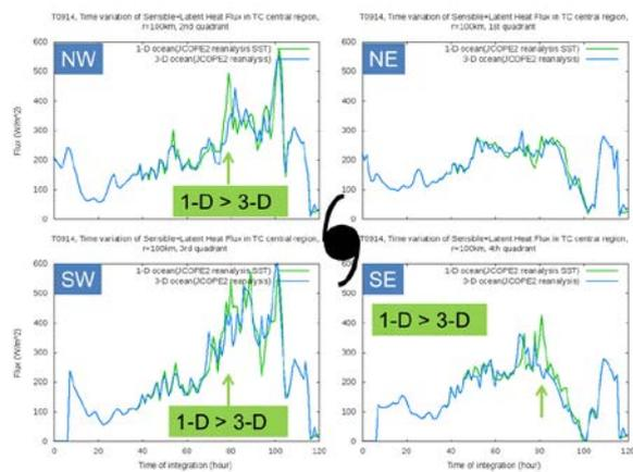
Figure 7. The time variation of sum of the sensible and latent heat fluxes averaged within 100 km radius around the TC center, divided into 4-quadrants for the coupled experiments with one-dimensional (green line) and three-dimensional (blue line) ocean, respectively.
