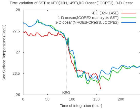
Figure 2. Time variation of the SST at the KEO buoy. Dotted line indicates the time of Choi-wan passing over the KEO buoy at 89 hour of the integration time (<http://www.pmel.noaa.gov/ocs/disdel/disdel.html>).
