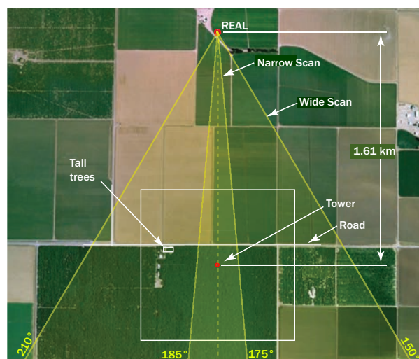
Figure 1: Plan view of the experimental area for the 2007 CHATS experiment. The REAL was located 1.61 km directly north of the 30-m tall NCAR ISFF tower. We limited our analysis to the 1 km 2 box centered on the tower.
