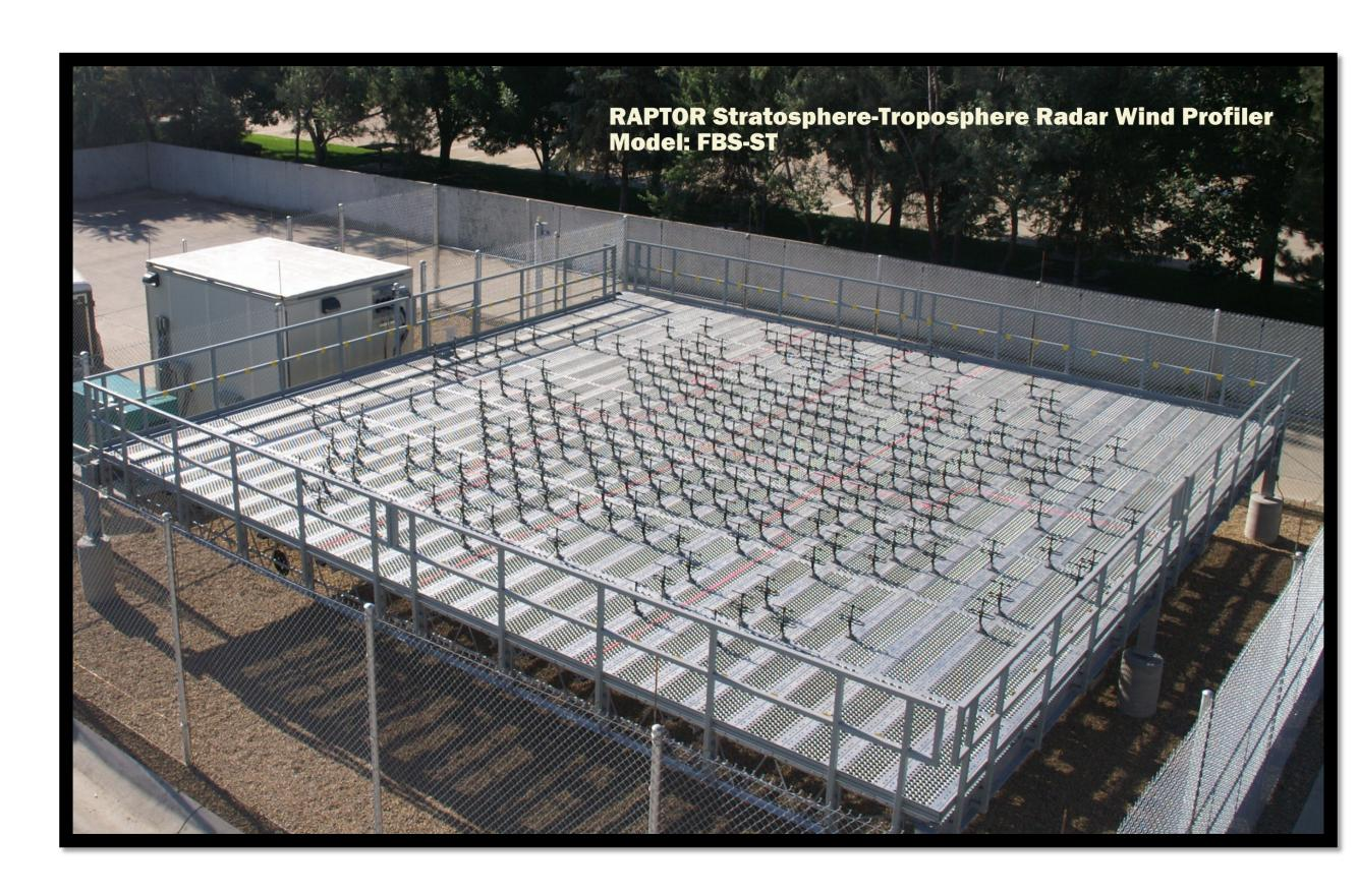
Technology is similar to the scalable DeTect, Inc. "full-size" **RAPTOR FBS-ST** model designed for National Weather Service (NWS), which uses up to a 12-kW transmitter and 11m x 11m antenna, and is designed for 16+ km height coverage.
