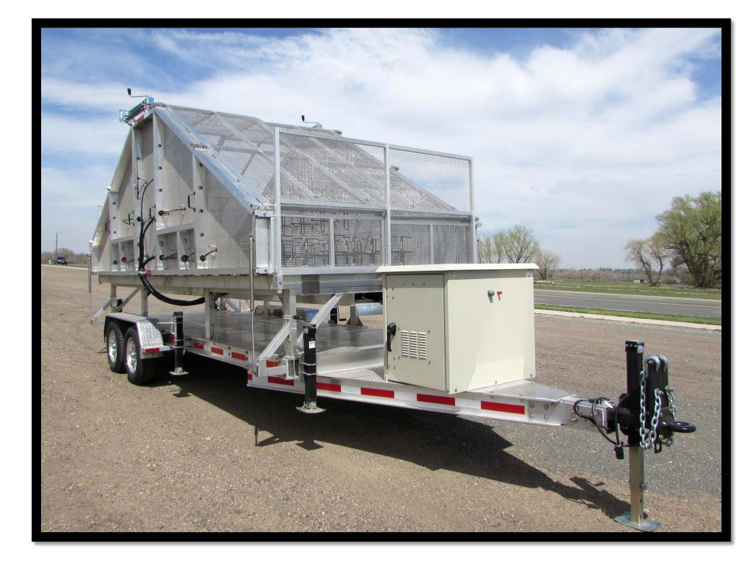
Antenna easily folds for simple transport and quick setup. Trailer can be pulled with standard full-size pickup. After leveling, only two cables are required to connect and begin operation of antenna.
