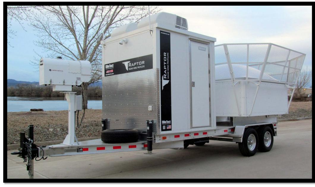
The **RAPTOR XBS-BL** is a "sister" system designed for boundary layer coverage, operating at 915 MHz or 1290 MHz. The 400-MHz band XBS-T (i.e., tropospheric) and 1-GHz band XBS-BL (i.e., boundary layer) share the same antenna pointing topology and other electronics. System is shown with integrated radiometer for humidity and temperature profiling.
