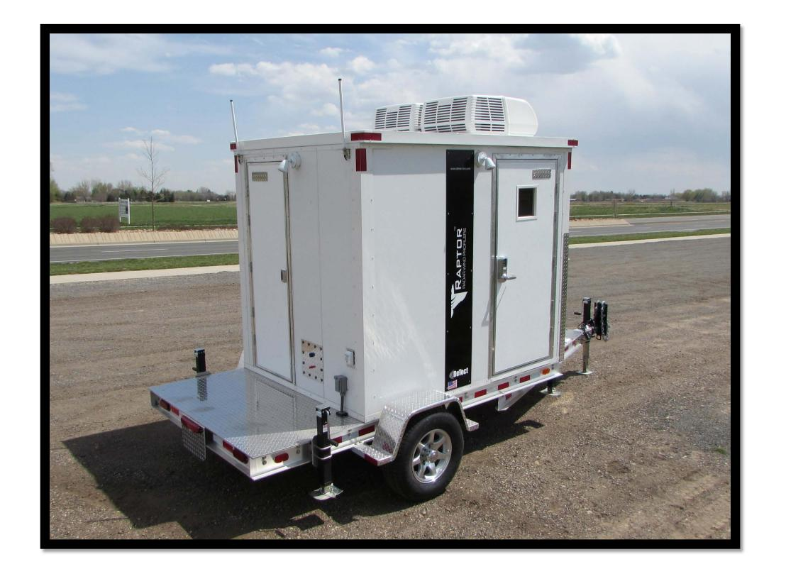
In mobile configuration, the electronics are shock-mounted in a 19" electronics rack on small trailer with air conditioning. Options include generator, cell-phone modem, met tower or integrated radiometer.
