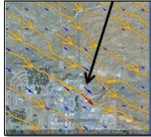
Figure 6. The diagnostic model output (blue) represents winds at 2.5-m AGL. The observation wind data sample is from 10-m AGL. The yellow lines are streamlines based on analysis of the model data. The black arrow flags the model-observation data area.
