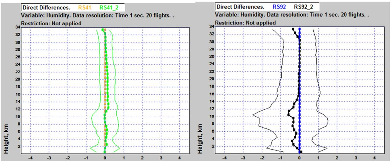
Figure 16. Reproducibility of daytime humidity measurement in Camborne campaign, RS41 on the left, RS92 on the right.
