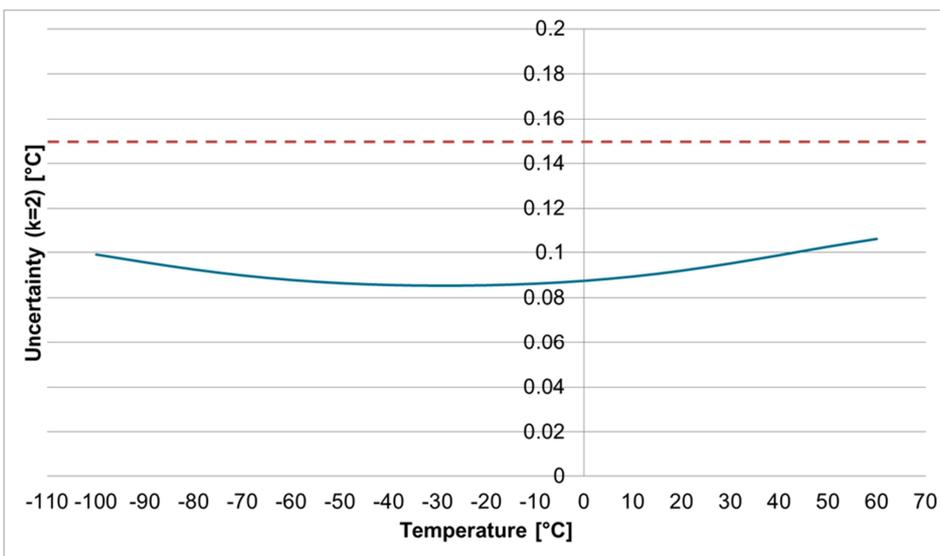
Figure 9. The combined uncertainty of the Vaisala Radiosonde RS41 temperature measurement after ground preparation (k=2). The dashed line indicates the calibration accuracy of RS92.
