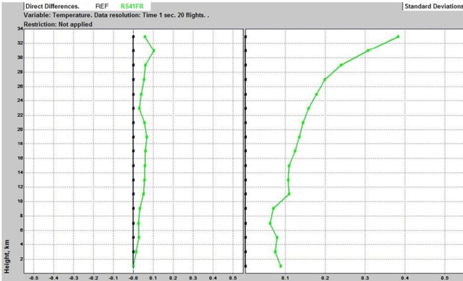
Figure 17. A twin-sounding comparison of RS41 temperature measurement against a multi-thermometer reference method – average temperature difference (left) and standard deviation of differences (right).
