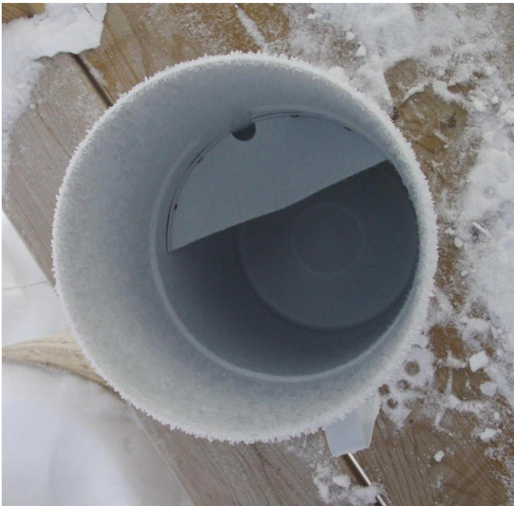
Figure 13: Frost on the R1 manual gauge (courtesy of P. Raczynski).
