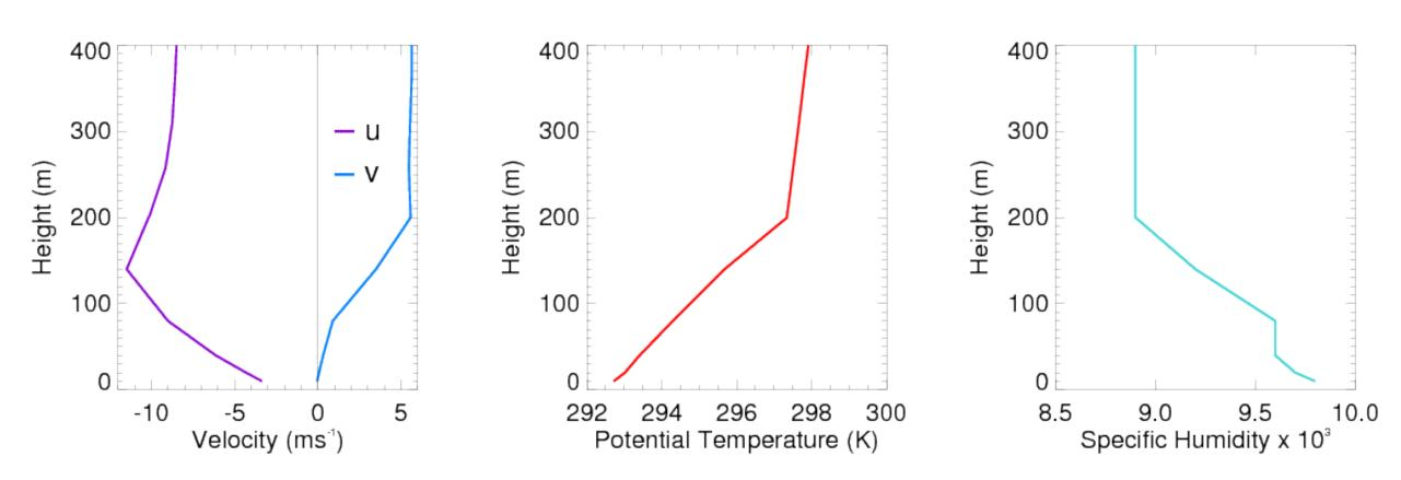
Initial profiles of wind, potential temperature and specific humidity.
