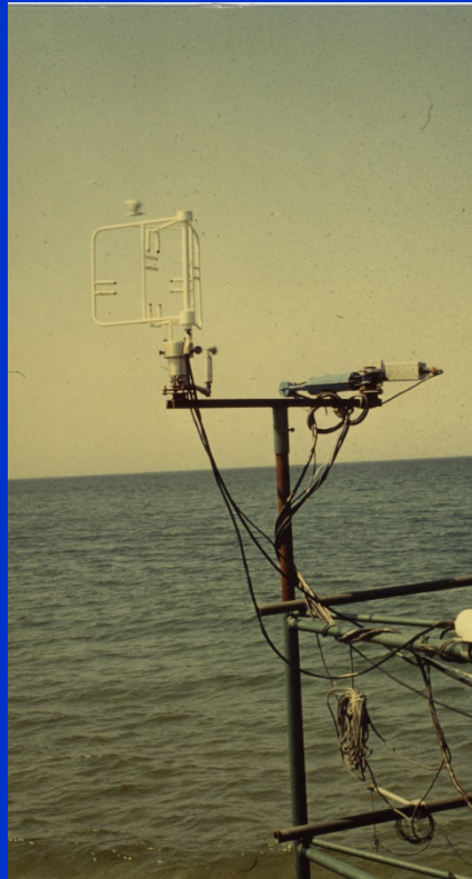
Sonic anemometers of the Meteorological Main Observatory Potsdam (Kaijo-Denki PAT) and of the Shirshov-Institute Moscow
