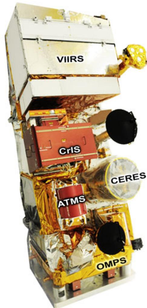
**Figure 5. Photo image of the NASA Suomi-NPP satellite with labels for the five sensors.** (<https://jointmission.gsfc.nasa.gov/cris.html>)
